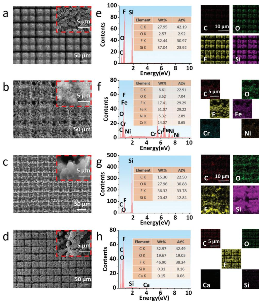
**Fig. 2** (a–d) SEM images of quartz glass, stainless steel, silicon wafer, and paper after femtosecond laser ablation; (e–h) EDS spectra and elemental mapping of laser-treated quartz glass, stainless steel, silicon wafer, and paper, respectively.
