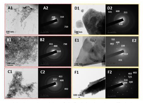
Fig. 3 High-resolution transmission electron microscopic images (series 1) and selected area electron diffraction images of  $PPy/MnO_2$  (series 2) recorded in a water/chloroform bisolvent medium at varying time intervals. The images A1 and A2, B1 and B2, C1 and C2, D1 and D2, E1 and E2, and F1 and F2 represent the reaction times of 2.5, 5, 7.5, 10, 12.5, and 15 hours, respectively.
