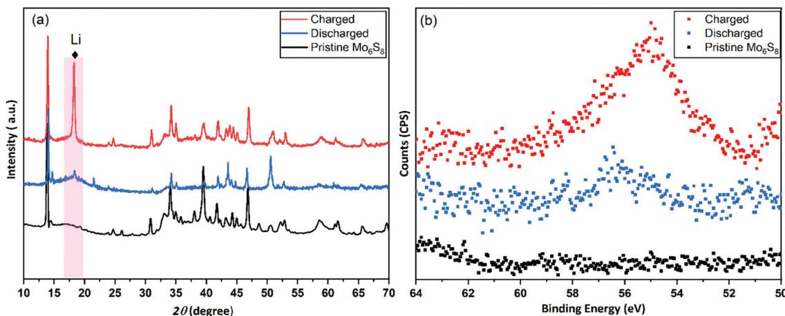
**Fig. 7** Post-mortem characterization on cycled  $\text{Mo}_6\text{S}_8$  electrodes. (a) Post-mortem P-XRD characterization was conducted on the pristine, fully charged to 2.2 V, and fully discharged to 0.5 V  $\text{Mo}_6\text{S}_8$  electrode. (b) High resolution XPS spectra of the Li 1s for the pristine, charged, and discharged  $\text{Mo}_6\text{S}_8$  electrode.
