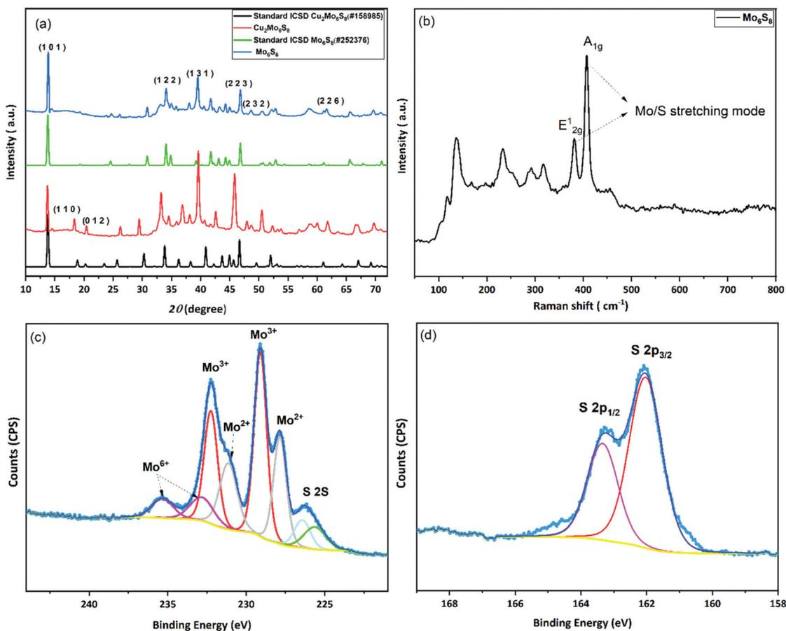
**Fig. 1** Characterization of the prepared materials: (a) P-XRD pattern of the as-synthesised  $\text{Cu}_2\text{Mo}_6\text{S}_8$  and  $\text{Mo}_6\text{S}_8$  along with their corresponding standard patterns, (b) Raman spectrum of  $\text{Mo}_6\text{S}_8$ , (c) high resolution XPS spectra of the Mo 3d/S 2s region and (d) S 2p region.
