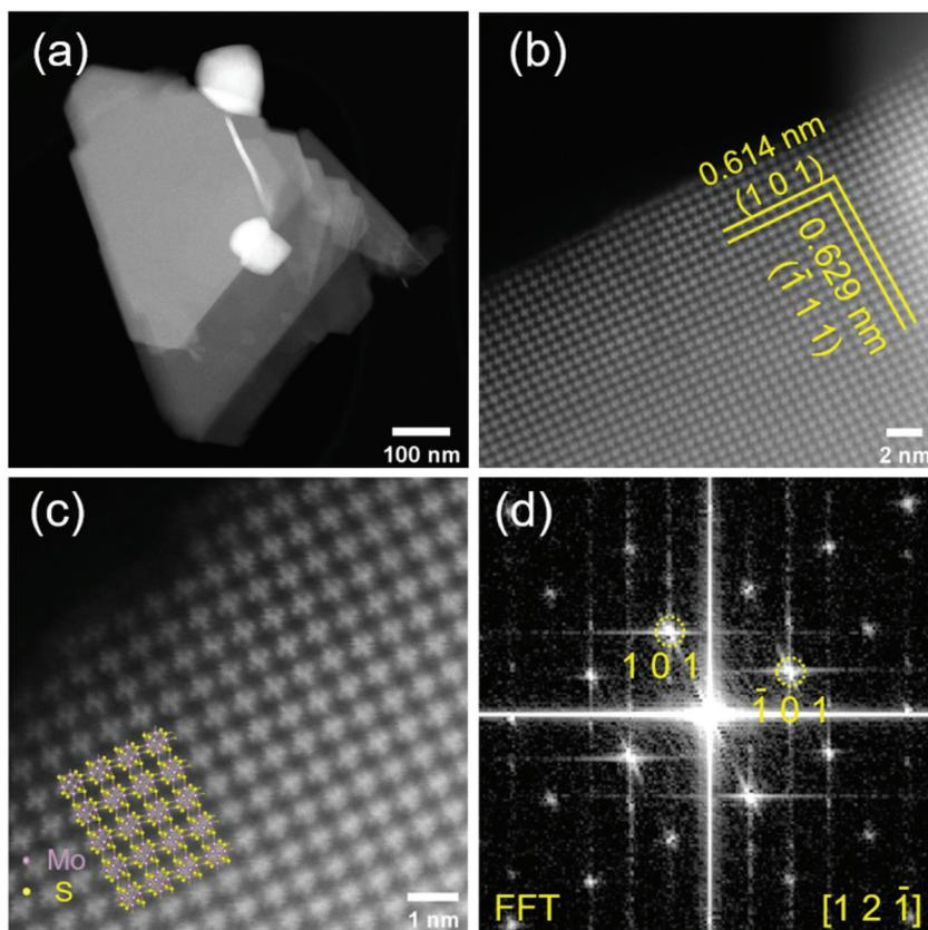
**Fig. 3** HAADF-STEM images of  $\text{Mo}_6\text{S}_8$  particle at low (a), medium (b) and high magnifications (c). The atomic resolution image in (c) reveals the expected crystal structure of  $\text{Mo}_6\text{S}_8$  viewed along  $[12\bar{1}]$  with an atomic model overlaid bottom left. (d) Fast Fourier Transform (FFT) obtained from (b) which can be indexed to the  $[12\bar{1}]$  zone-axis of  $\text{Mo}_6\text{S}_8$ .
