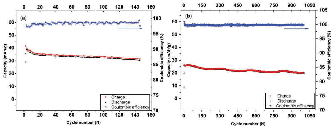
Fig. 6 Long-term cycling performance and coulombic efficiency of Mo<sub>6</sub>S<sub>8</sub> nanocubes at 0.2 C-rate (a), and 4 C-rate (b).
