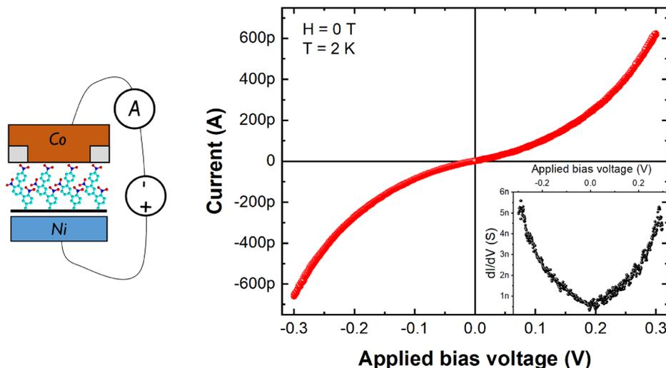
**Fig. 3** Charge transport characteristics.  $I$ - $V$  and  $dI/dV$  (inset) of a junction measured across a Ni/Gr/NB (1.3 nm)/Co junction at 2 K revealing high electrical resistance and non-linear tunneling characteristics. A schematic of the measurement configuration is shown on the left.
