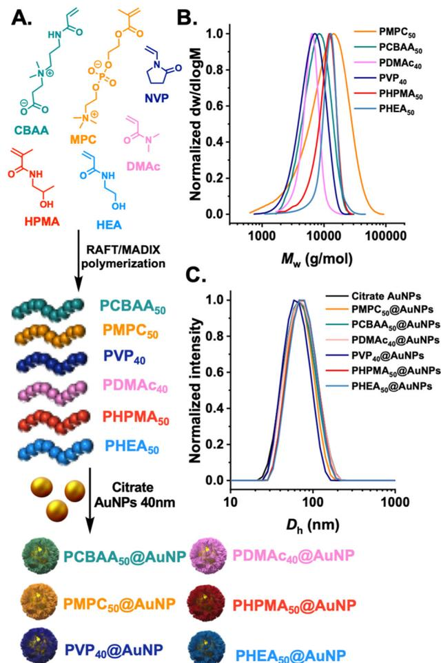
**Fig. 1** Synthesis of polymer-tethered gold nanoparticles. (A) Polymers synthesised in this study. Subscript denotes the targeted degree of polymerisation; (B) size exclusion chromatography of the polymer library; (C) dynamic light scattering of citrate AuNPs (40 nm) and with polymers tethered to their surface.
