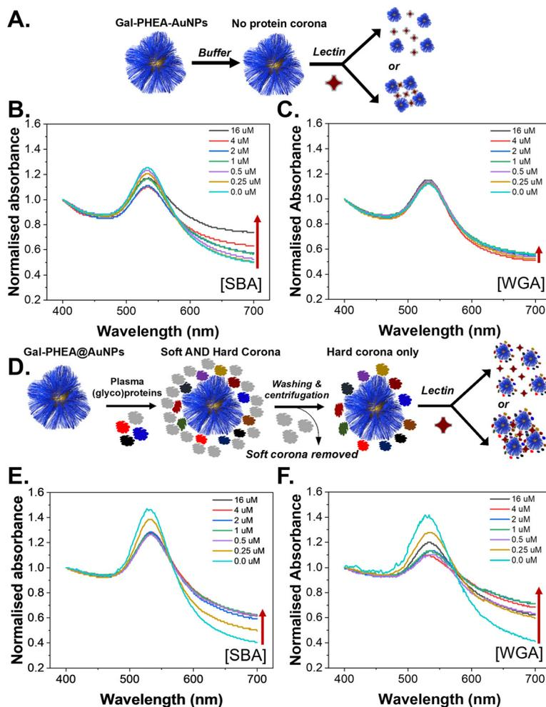
**Fig. 4** Effect of hard corona on lectin binding capacity to Gal-PHEA<sub>25</sub>@AuNPs. (A) Schematic of aggregation assay in buffer only; (B) UV-Vis spectra versus SBA in buffer; (C) UV-vis spectra versus WGA in buffer; (D) schematic of hard corona formation and aggregation assay; (E) UV-Vis spectra versus SBA with hard corona; (F) UV-Vis spectra versus WGA with hard corona.
