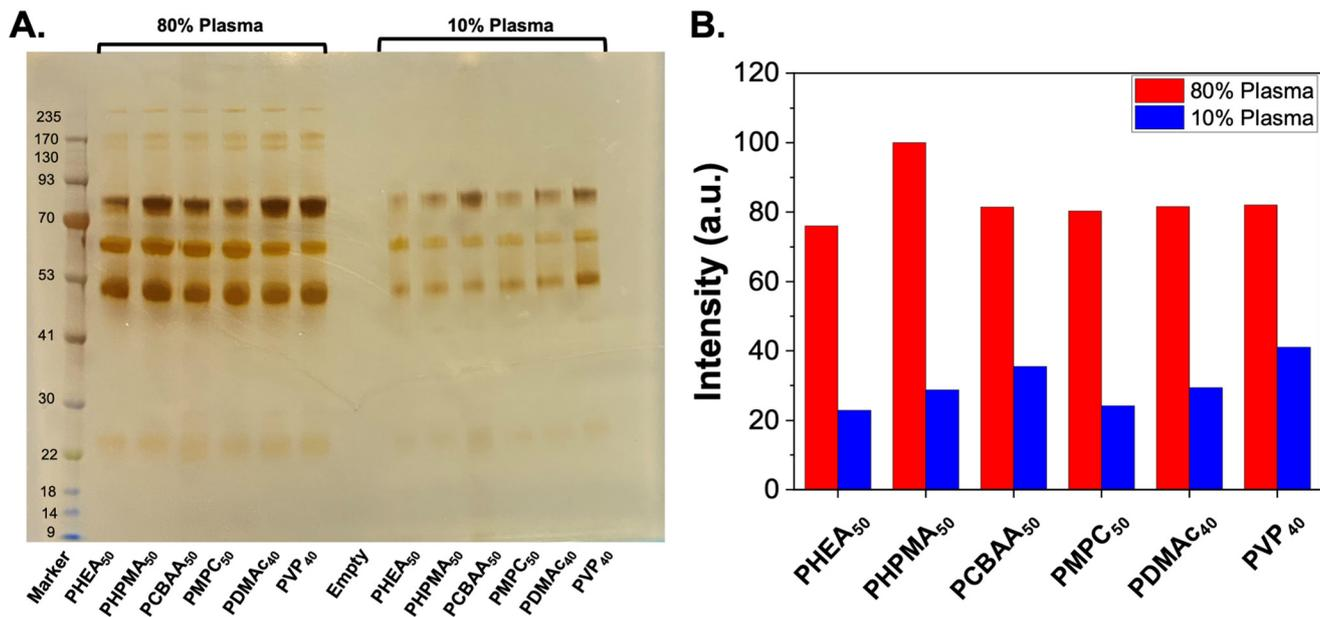
**Fig. 2** SDS-PAGE of protein corona formation on polymer-coated gold nanoparticles. (A) Silver-stained gel showing hard corona proteins released from nanoparticles after incubation with bovine plasma. (B) Densitometry analysis of gel. Polymer codes refer to polymer coatings (Fig. 1) on 40 nm gold particles.
