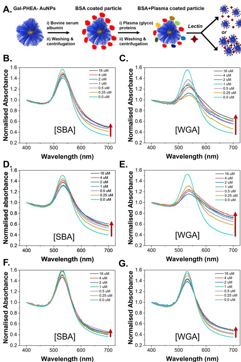
**Fig. 10** Lectin binding by aggregation assay against nanoparticles pre-blocked with BSA, before exposure to plasma. (A) Schematic of experimental process; (B) Gal-PHEA<sub>25</sub>@AuNP<sub>40</sub> versus SBA; (C) Gal-PHEA<sub>25</sub>@AuNP<sub>40</sub> versus WGA; (D) Gal-PHEA<sub>50</sub>@AuNP<sub>40</sub> versus SBA; (E) Gal-PHEA<sub>50</sub>@AuNP<sub>40</sub> versus WGA; (F) Gal-PHEA<sub>75</sub>@AuNP<sub>40</sub> versus SBA; (G) Gal-PHEA<sub>75</sub>@AuNP<sub>40</sub> versus WGA.
