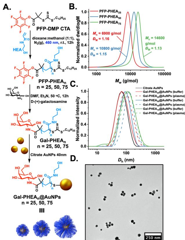
**Fig. 3** Glyconanoparticle synthesis. (A) Synthetic scheme for the synthesis of PFP-terminated PHEA, functionalisation with galactosamine and immobilisation onto gold nanoparticles; (B) size exclusion chromatography analysis of PHEA's; (C) dynamic light scattering of polymer-coated particles in buffer and in plasma; (D) representative TEM of polymer-coated nanoparticles. AuNPs = 40 nm in all cases.
