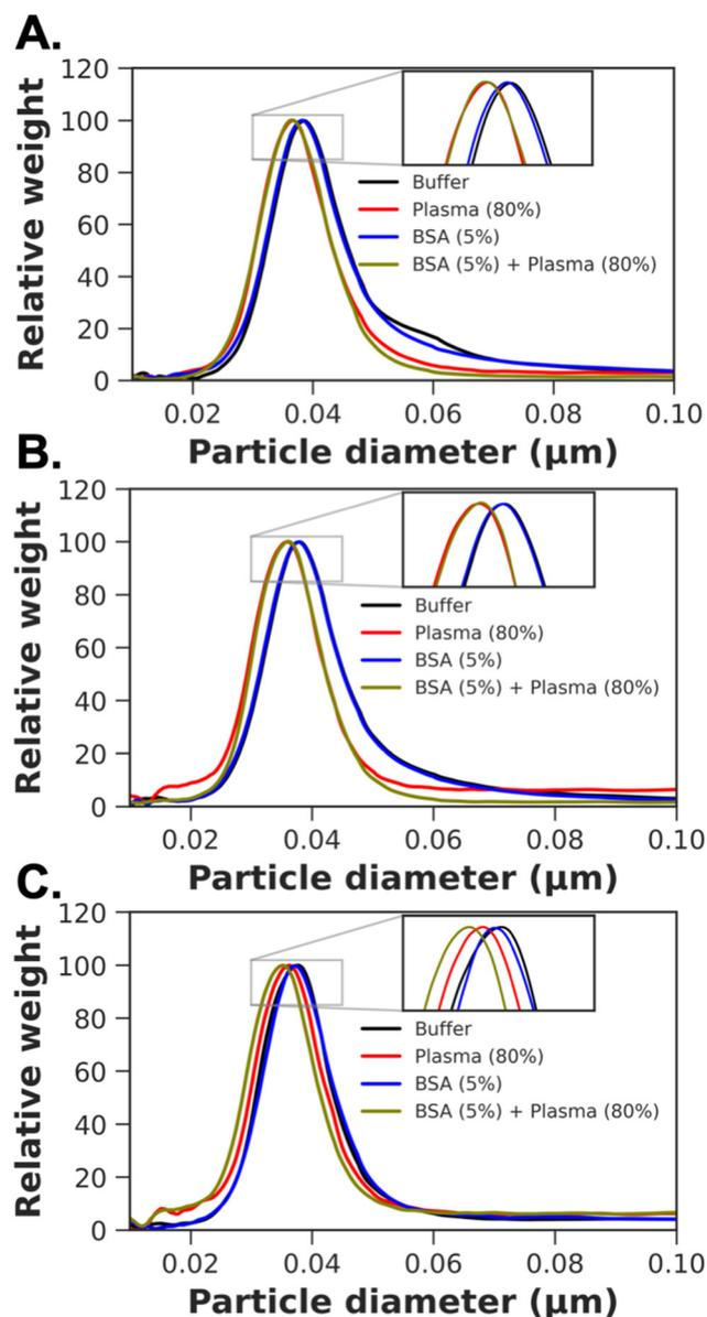
Fig. 9 Differential centrifugation sedimentation analysis of particles, in buffer, plasma, BSA, or BSA then plasma. (A) Gal-PHEA<sub>25</sub>@AuNP<sub>40</sub>; (B) Gal-PHEA<sub>50</sub>@AuNP<sub>40</sub>; (C) Gal-PHEA<sub>75</sub>@AuNP<sub>40</sub>.
