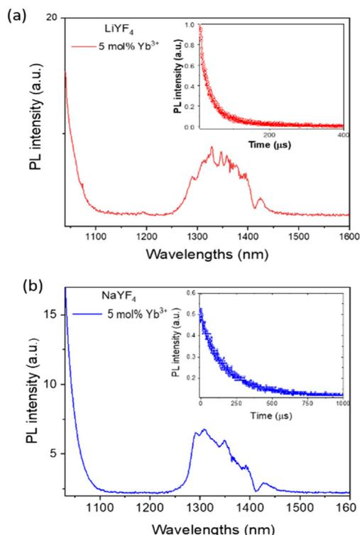
Fig. 5 NIR-II PL spectra of  $\text{LiYF}_4:\text{Pr}^{3+}/\text{Yb}^{3+}$  (a) and  $\text{NaYF}_4:\text{Pr}^{3+}/\text{Yb}^{3+}$  (b) NCs in  $\text{CHCl}_3$ . Insets of a and b show corresponding DCL decays acquired at 1320 nm under 980 nm excitation.
