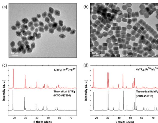
Fig. 2 Selected TEM images of (a) LiYF<sub>4</sub>:Pr<sup>3+</sup>/Yb<sup>3+</sup> and (b) NaYF<sub>4</sub>:Pr<sup>3+</sup>/Yb<sup>3+</sup> NCs. The corresponding PXRD patterns of (c) LiYF<sub>4</sub>:Pr<sup>3+</sup>/Yb<sup>3+</sup> and (d) NaYF<sub>4</sub>:Pr<sup>3+</sup>/Yb<sup>3+</sup> NCs versus theoretical patterns from the database.
