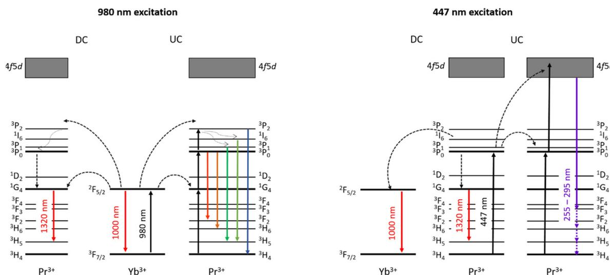
**Fig. 1** A scheme of electronic levels and transitions corresponding to VIS-to-UVC UCL and NIR-to-NIR-II DCL processes in  $\text{Pr}^{3+}$  and  $\text{Yb}^{3+}$  in fluoride NCs. The UCL and DCL mechanisms are illustrated under (a) 980 nm laser excitation for visible and NIR emissions and (b) 447 nm laser excitation for UVC and NIR emissions.
