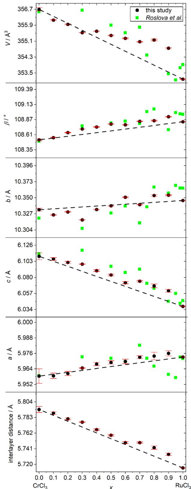
Fig. 4 Refined unit cell parameters of  $\text{Cr}_{1-x}\text{Ru}_x\text{Cl}_3$  compared to values of Roslova *et al.*<sup>25</sup> and Vegard's law. Error bars are estimated standard deviations derived from the refinement software.
