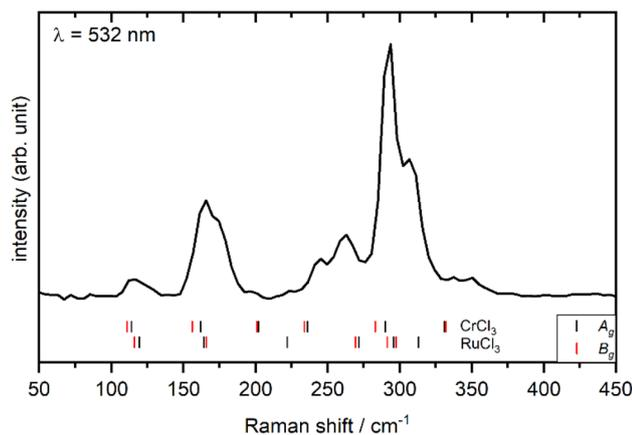
**Fig. 8** Raman spectrum of a nanocrystal with  $x = 0.4$  compared to reference peaks for the parent compounds  $\text{CrCl}_3$ <sup>26</sup> and  $\text{RuCl}_3$ <sup>27</sup>.
