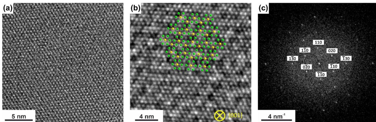
**Fig. 7** HRTEM investigations on as-grown  $\text{CrCl}_3$ - $\text{RuCl}_3$  nanoflakes: (a) HRTEM image recorded along [001] zone axis of the monoclinic lattice. (b) Image at higher magnification as (a) but at the same crystal orientation with overlaid atomic model (Ru/Cr – yellow, Cl – green). (c) Fourier transformed image (a) with some of the reflections indexed.
