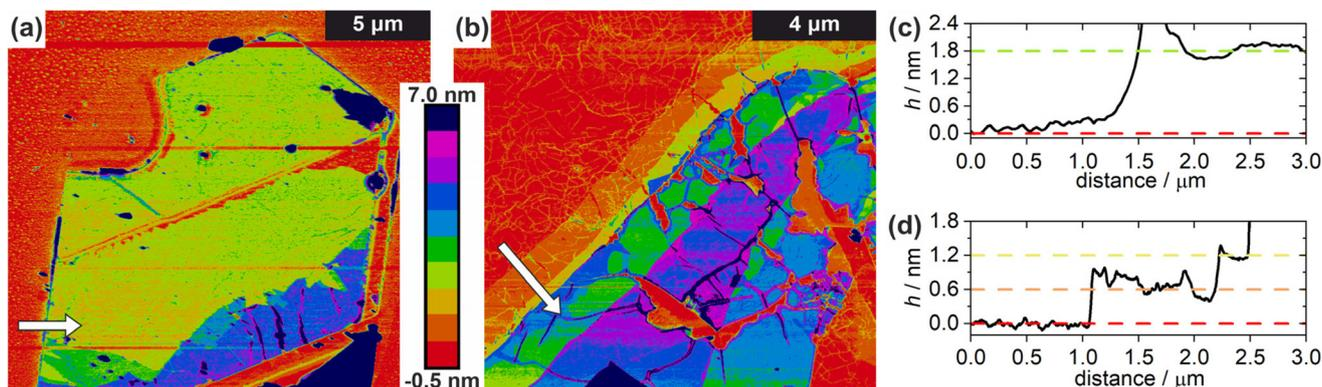
**Fig. 10** AFM measurements of few-layer structures produced by delamination: (a) large area trilayer crystal, (b) structure with stacked mono- and bilayer areas on the edge. (c + d) height profiles of the steps in (a) and (b) marked by the white arrow.
