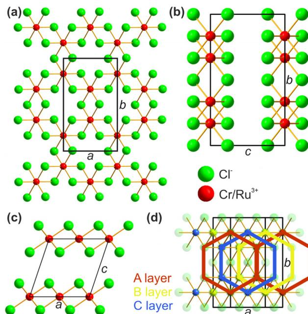
**Fig. 3** Crystal structure of  $\text{CrCl}_3$  and  $\text{RuCl}_3$ : (a) view onto a single [001] plane, (b) side view along the  $a$ -axis, (c) side view along the  $b$ -axis, (d) top view upon multiple [001] planes with highlighted stacking direction along the  $a$ -axis.
