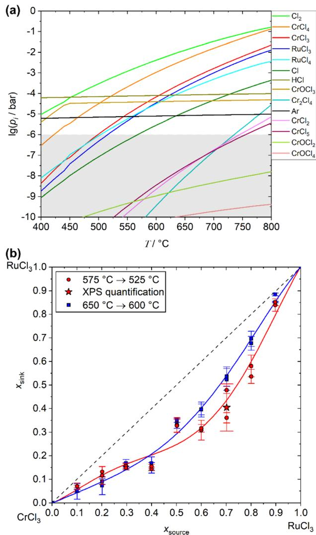
**Fig. 5** (a) Calculated partial pressures of known vapour species over a  $\text{Cr}_{1-x}\text{Ru}_x\text{Cl}_3$  sample with  $x = 0.5$  including traces of  $\text{H}_2\text{O}$  and Ar. The grey area indicates pressures that are too low for transport relevance. (b) Observed values of  $x$  of deposited crystals in the sink. Solid lines are only added to guide the eye. Error for EDX measurements is the standard deviation. Error for XPS measurement estimated with 0.1.
