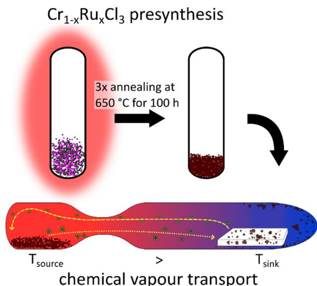
**Fig. 1** Schematic illustration of the synthesis processes. Homogeneous solid solution powder is synthesized by repeated tempering of  $\text{CrCl}_3$  and  $\text{RuCl}_3$ . This is then used as starting material for CVT experiments to deposit nanocrystals directly on a substrate.
