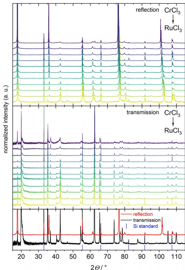
**Fig. 2** Normalized, background subtracted and stacked powder XRD pattern of the  $\text{Cr}_{1-x}\text{Ru}_x\text{Cl}_3$  solid solution series in steps of 10 mol%, measured in (a) reflection and (b) transmission geometry. (c) Comparison of observable peaks between reflection (red) and transmission (black) geometry for the same  $x = 0.5$  sample.
