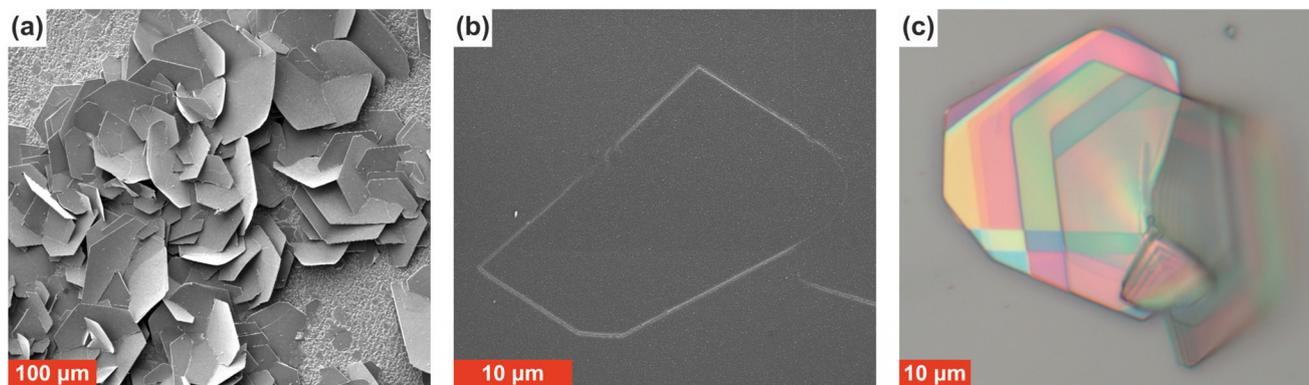
**Fig. 6** SEM image of (a) non-epitaxial grown crystal agglomerates and (b) a single as-grown nanosheet of about 30 nm in height (visible surface particles and cracks caused by carbon sputtering). (c) Microscope image of a microcrystal showing layer steps of a few nanometres distinguishable by colour.
