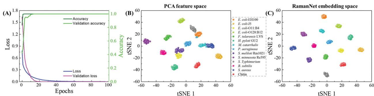
**Fig. 7** (A) Loss during training the RamanNet model. Although the model was trained for 100 epochs, it achieves convergence within 40 epochs. Dimensionality reduction using RamanNet. The 256-dimensional feature space is projected into a 2 dimensional-map using t-SNE: (B) PCA and (C) RamanNet.
