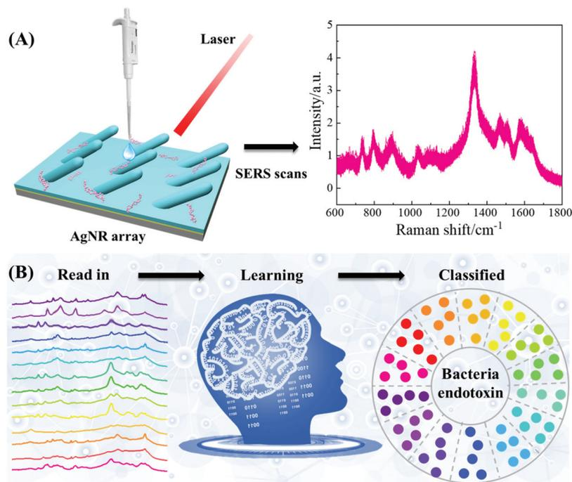
**Fig. 1** The general schematic strategy for the classification of bacterial endotoxins using SERS and MLAs. (A) Sample preparation and SERS measurements and (B) spectral pre-processing and classification using an MLA.
