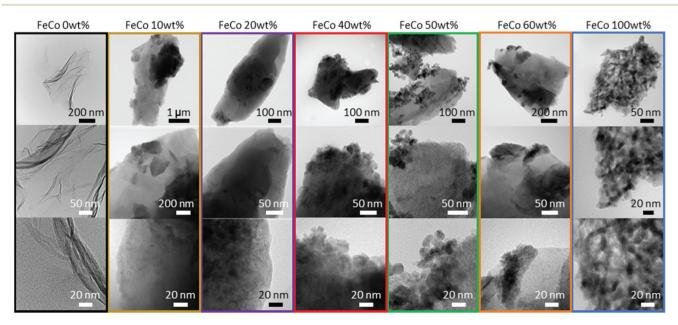
Fig. 4 TEM micrographs in increasing magnification from the top to bottom of FeCo 0 wt% (black), FeCo 10 wt% (brown), FeCo 20 wt% (purple), FeCo 40 wt% (red), FeCo 50 wt% (green), FeCo 60 wt% (orange), and FeCo 100 wt% (blue) samples.
