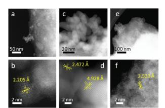
Fig. 7 STEM-HAADF images of FeCo 40 wt%, top showing low magnification images and bottom showing high magnification images. (a–d) Areas with the presence of well-defined nanoparticles. (e and f) Area without well-defined particles. (b) Lattice spacing of a CoO particle. (d) Lattice spacings of CoO (left) and CoFe<sub>2</sub>O<sub>4</sub> (right) particles. (f) Lattice spacings of CoFe<sub>2</sub>O<sub>4</sub> on the surface of rGO.
