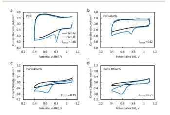
Fig. 10 CVs of (a) a Pt/C reference, (b) FeCo 0 wt%, (c) FeCo 40 wt% and (d) FeCo 100 wt% in a saturated Ar electrolyte (black line) and a saturated  $O_2$  electrolyte (blue line). Scan rate was 50 mV s<sup>-1</sup>, in 1.0 M KOH with a stationary RDE.
