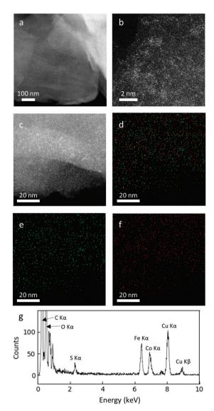
Fig. 6 STEM micrographs of FeCo 10 wt%. (a-c) HAADF images at various magnifications. (c) Area used for EDS element mapping. (d) Overlay of Fe K (red) and Co K (green). (e) Element map for Co K (green). (f) Element map for Fe K (red). (f). (g) EDS spectrum of the mapped area.
