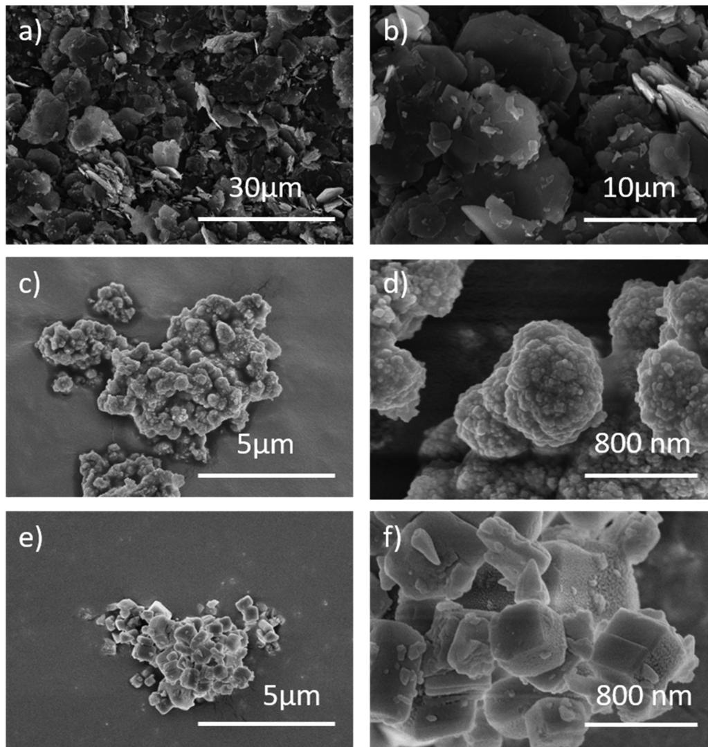
**Fig. 2** (a and b) SEM images of NVPFO<sub>2</sub>-Iono. (c and d) SEM-FEG images of NVPFO<sub>2</sub>-Nano. (e and f) SEM-FEG images of NVPFO<sub>2</sub>-Bulk.
