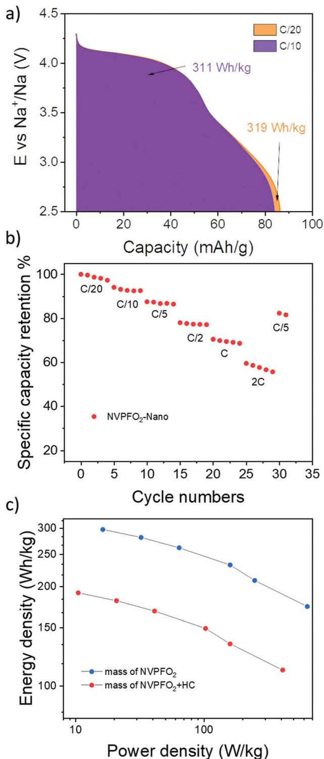
Fig. 12 (a) Energy density calculated for NVPFO<sub>2</sub>-Nano at C/20 and C/10. (b) Specific capacity retention in % upon increasing the C-rate. (c) Ragone plots of the NVPFO<sub>2</sub>-Nano full cell; the blue points correspond to the capacity calculated based on the NVPFO<sub>2</sub> mass and the red points on both electrode masses.
