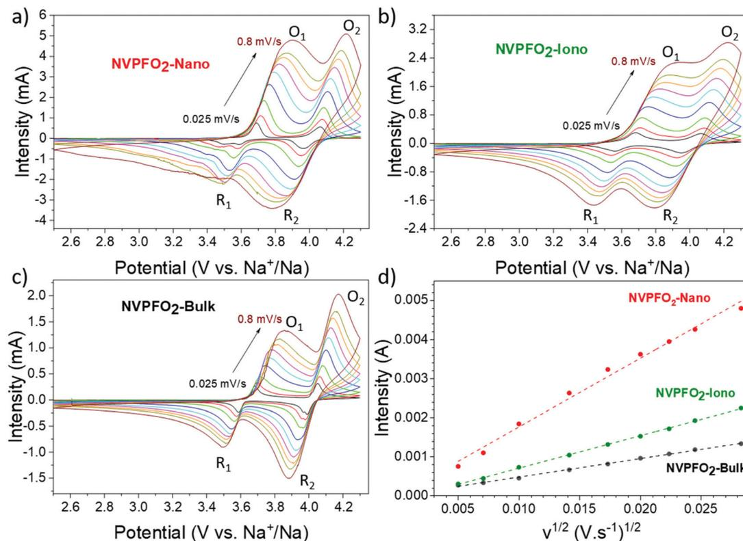
**Fig. 10** (a–c) CV curves at different scan rates and (d) the corresponding linear fitting curves between the maximum current ( $i_p$ ) and the square root of the scan rate ( $v^{1/2}$ ) for the  $O_1$  peak of each compound.
