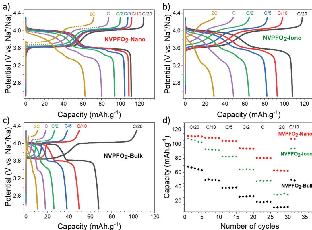
Fig. 6 (a–c) Charge and discharge curves of all the NVPFO<sub>2</sub> materials at different cycling rates. (d) Rate capabilities obtained for all these materials, from C/20 to 2C.
