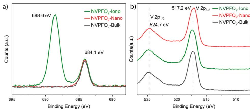
Fig. 4 (a) F 1s XPS spectra and (b) V 2p XPS spectra for all the NVPFO<sub>2</sub> materials.
