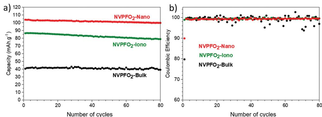
**Fig. 11** (a) Evolution of reversible capacity upon long-term cycling at C/5 and (b) related coulombic efficiency of all the NVPFO<sub>2</sub> materials.
