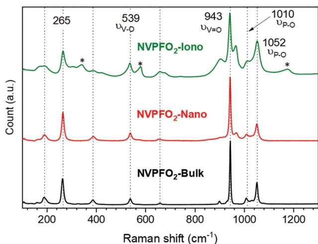
Fig. 3 Raman spectra of NVPFO<sub>2</sub>-Iono (green), NVPFO<sub>2</sub>-Nano (red) and NVPFO<sub>2</sub>-Bulk (black). The band marked with a star on the Raman spectrum corresponds to the EMI TFSI ionic liquid.
