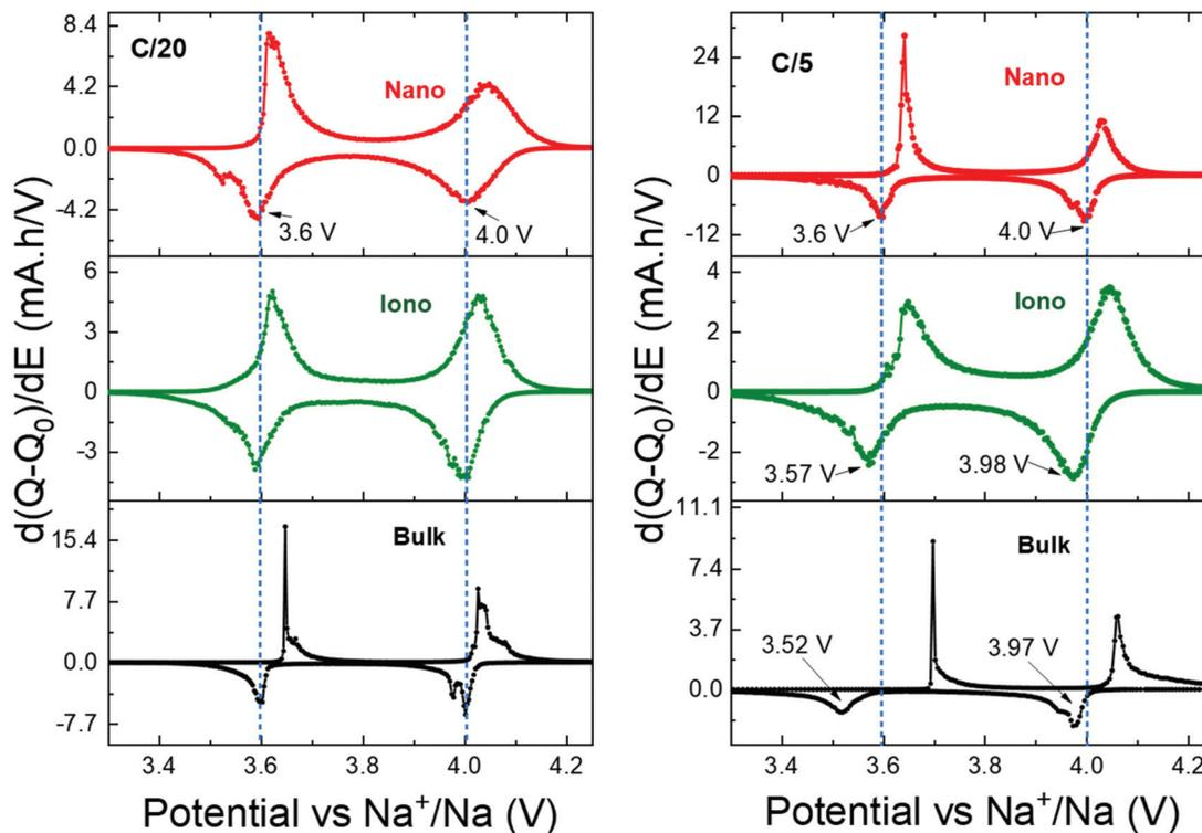
Fig. 7 First derivative curves of the second cycle of galvanostatic charge discharge process of all the NVPFO<sub>2</sub> materials at C-rates of C/20 and C/5.
