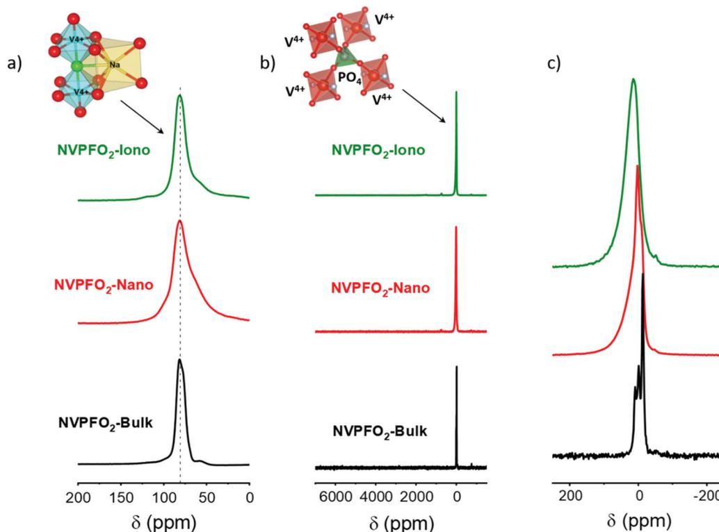
Fig. 5 (a) <sup>23</sup>Na solid-state MAS NMR spectra of NVPFO<sub>2</sub>-Iono (green), NVPFO<sub>2</sub>-Nano (red) and NVPFO<sub>2</sub>-Bulk (black). (b) Corresponding <sup>31</sup>P solid-state MAS NMR spectra. (c) Enlargement of the signals around 0 ppm.
