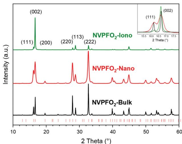
Fig. 1 X-ray diffraction patterns of NVPFO<sub>2</sub>-Iono (green curve), NVPFO<sub>2</sub>-Nano (red curve) and NVPFO<sub>2</sub>-Bulk (black curve). The red ticks correspond to theoretical positions as reported in ICDD 01-083-7199. The inset shows the enlargement of the (111) and (002) reflections.
