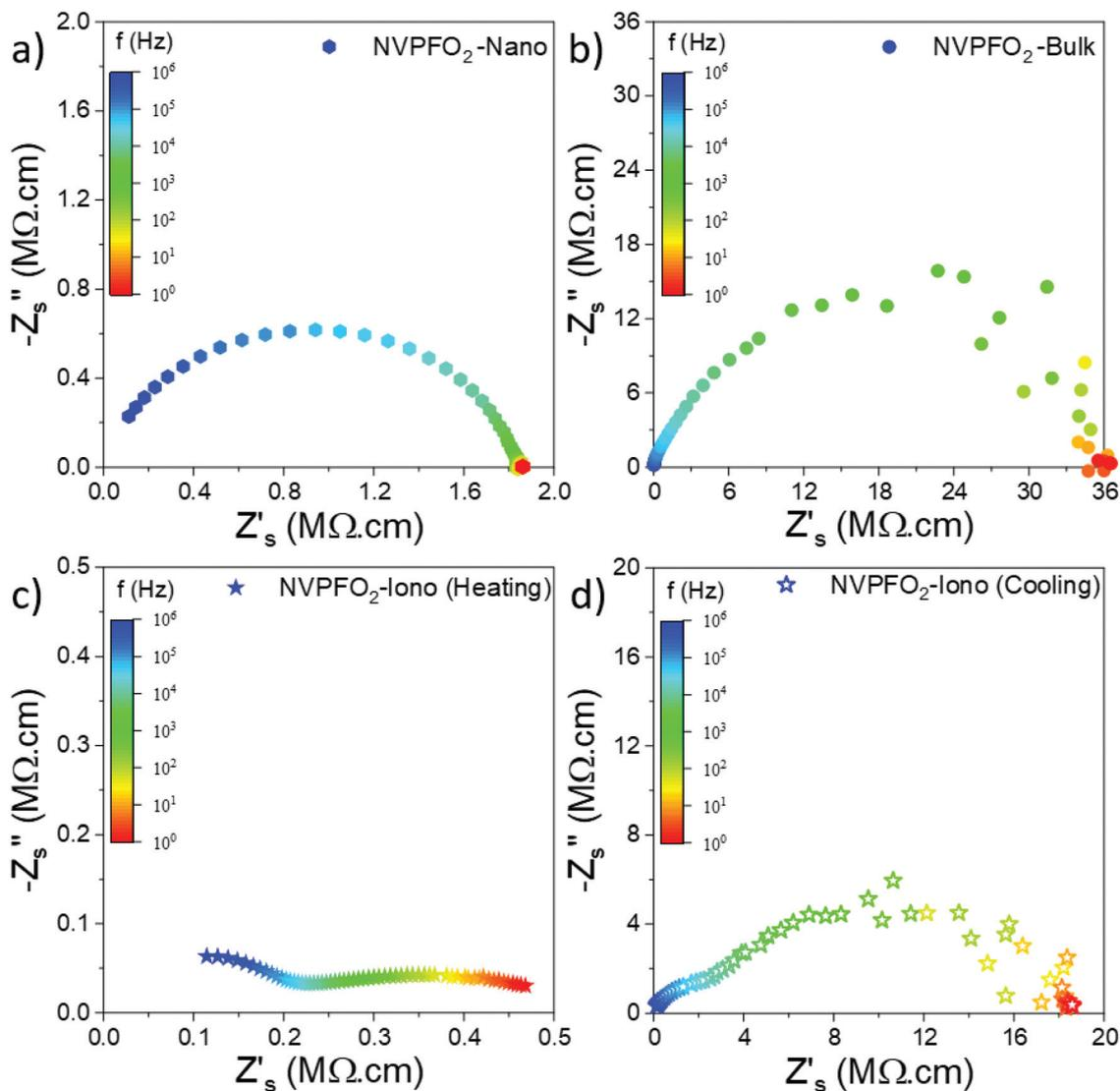
**Fig. 8** EIS analyses of  $\text{Na}_3\text{V}_2(\text{PO}_4)_2\text{FO}_2$  samples recorded at 200 °C under heating for NVPFO<sub>2</sub>-Nano (a) and NVPFO<sub>2</sub>-Bulk (b) as well as for NVPFO<sub>2</sub>-Iono under heating (c) and under cooling (d). The complex impedance data shown here have already been normalized regarding the shape factor of each sample for comparison purposes.
