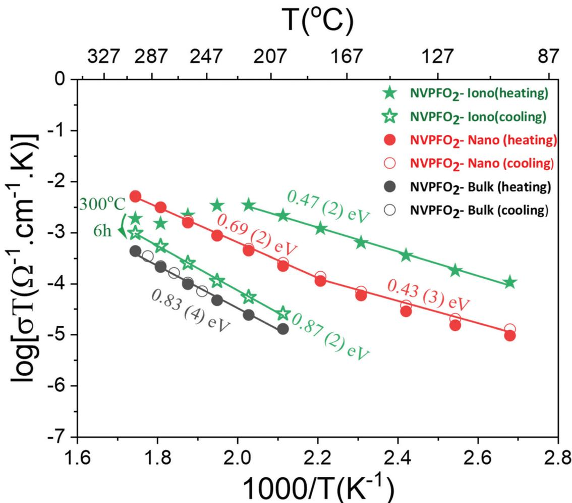
Fig. 9 Arrhenius-like plots of the dependence of the overall electric conductivity on the inverse temperature for NVPFO<sub>2</sub> samples synthesized under different conditions.
