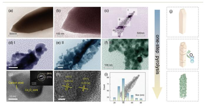
Fig. 3 TEM and HR-TEM images of (a), (b) ZIF-67, (c-h) Co<sub>3</sub>O<sub>4</sub>/C. Inset in (g) is the corresponding SAED pattern. (i) Size distribution of Co<sub>3</sub>O<sub>4</sub>/C nanoparticles. (j) Schematic illustration for the pyrolysis from ZIF-67 to Co<sub>3</sub>O<sub>4</sub>/C.
