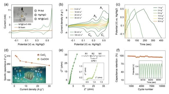
Fig. 8 (a) CV curves of Ni foam and NF@Co/C-550 sample at a scan rate of 5 mV s $^{-1}$ . Inset is a three-electrode system. (b) CV curves of NF@Co/C-550 sample at different scan rates. (c) GCD curves at different current densities. (d) Specific capacitance. Inset is the schematic illustration for electrode reaction. (e) Nyquist plots and the corresponding equivalent circuit. (f) Cycling performance at a charge–discharge current density of 10 A  $q^{-1}$ .
