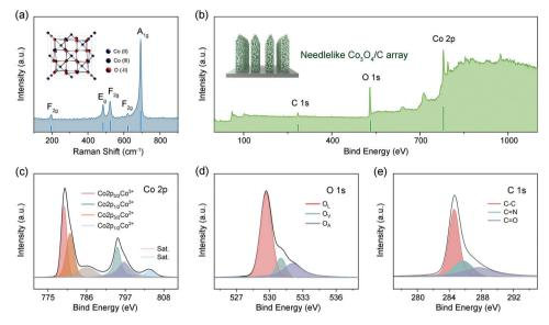
Fig. 4 (a) Raman spectrum of NF@Co/C, and inset is the crystal structure of Co<sub>3</sub>O<sub>4</sub>. (b) Broad scan XPS spectrum of NF@Co/C, and inset is the corresponding model. (c) Co 2p spectrum. (d) O 1s spectrum. (e) C 1s spectrum.
