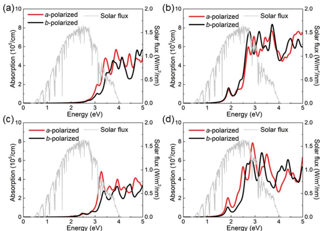
Fig. 8 Absorption spectrum of (a) GeS, (b) GeSe, (c) SiS and (d) SiSe monolayers, respectively. The red and black lines denote the absorption of *a*-polarized and *b*-polarized light, respectively.
