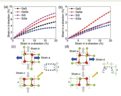
Fig. 7 (a) Strain in the b-direction under the external uniaxial a-direction strain and (b) the strain in the a-direction under the external uniaxial b-direction strain of the GeS, GeSe, SiS and SiSe monolayers; the schematic diagram of thickness deformation by the strain along the (c) a-direction and (d) b-direction of the MX monolayers; here the loading strain is shown in blue, while the induced strain is shown in grey.
