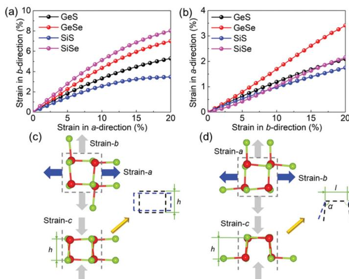
**Fig. 7** (a) Strain in the *b*-direction under the external uniaxial *a*-direction strain and (b) the strain in the *a*-direction under the external uniaxial *b*-direction strain of the GeS, GeSe, SiS and SiSe monolayers; the schematic diagram of thickness deformation by the strain along the (c) *a*-direction and (d) *b*-direction of the MX monolayers; here the loading strain is shown in blue, while the induced strain is shown in grey.
