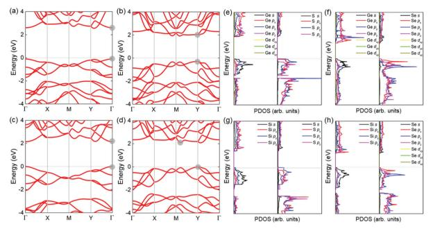
Fig. 5 Band structure of the monolayer (a) GeS, (b) GeSe, (c) SiS and (d) SiSe calculated by the HSE06 method, and the partial density of states of the monolayer (e) GeS, (f) GeSe, (g) SiS and (h) SiSe calculated by PBE. In (a–d), the locations of the CBM and VBM are marked by grey dots.
