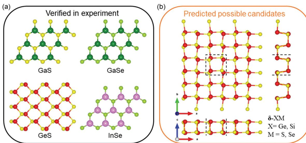
Fig. 1 (a) Synthesized IV–VI monolayers in a previous experiment and (b) crystal structure of the newly predicted  $\delta$ -IV–VI monolayers  $XM$  ( $X = Ge$  and  $Si$ ;  $M = S$  and  $Se$ ). The yellow and red balls are  $M$  and  $X$  atoms, respectively.
