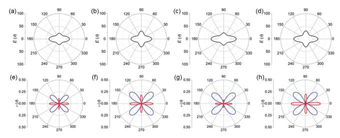
Fig. 6 Young's modulus of the (a) GeS, (b) GeSe, (c) SiS and (d) SiSe monolayers; the Poisson ratios of the (e) GeS, (f) GeSe, (g) SiS and (h) SiSe monolayers, respectively. The blue and red lines represent the positive and negative values.
