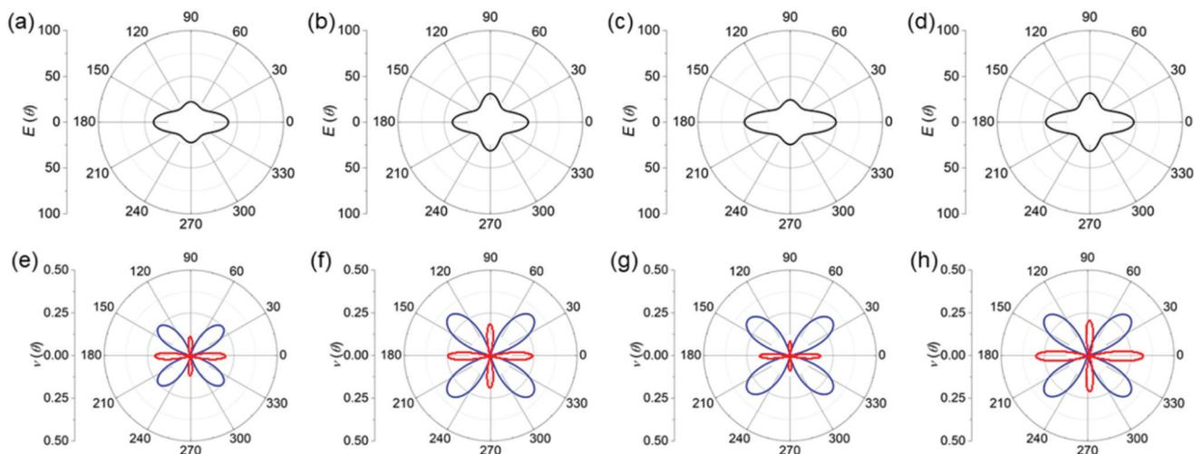
**Fig. 6** Young's modulus of the (a) GeS, (b) GeSe, (c) SiS and (d) SiSe monolayers; the Poisson ratios of the (e) GeS, (f) GeSe, (g) SiS and (h) SiSe monolayers, respectively. The blue and red lines represent the positive and negative values.
