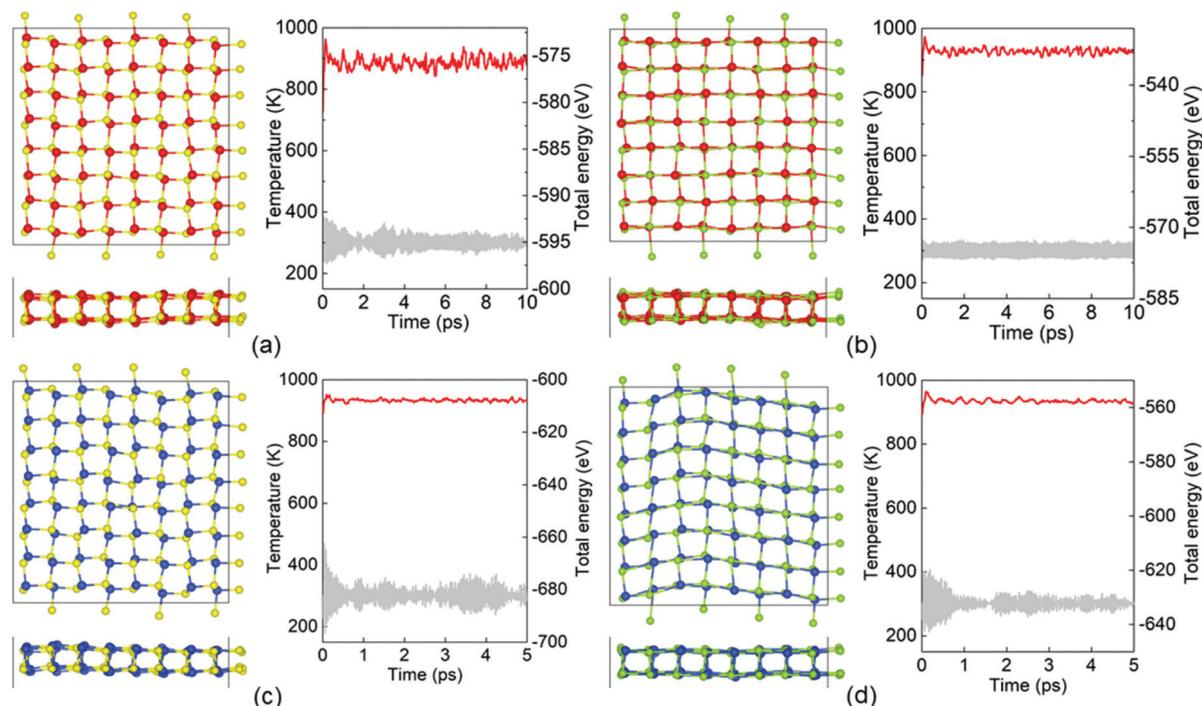
Fig. 4 Total energy and the temperature fluctuation of the (a) GeS, (b) GeSe, (c) SiS and (d) SiSe monolayers during the AIMD simulation, the insets are the atomic structure after 5 ps at 300 K. The red, yellow, cyan and blue marks represent the Ge, S, Se and Si atoms, respectively; the red and gray lines represent the system total energy and temperature calculated by the AIMD simulation.
