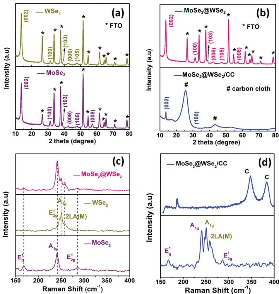
Fig. 3 XRD pattern (a) WSe<sub>2</sub> and MoSe<sub>2</sub> (b) MoSe<sub>2</sub>@WSe<sub>2</sub>/FTO and MoSe<sub>2</sub>@WSe<sub>2</sub>/CC. Raman spectra (c) WSe<sub>2</sub> and MoSe<sub>2</sub> (d) MoSe<sub>2</sub>@WSe<sub>2</sub>/FTO and MoSe<sub>2</sub>@WSe<sub>2</sub>/CC.
