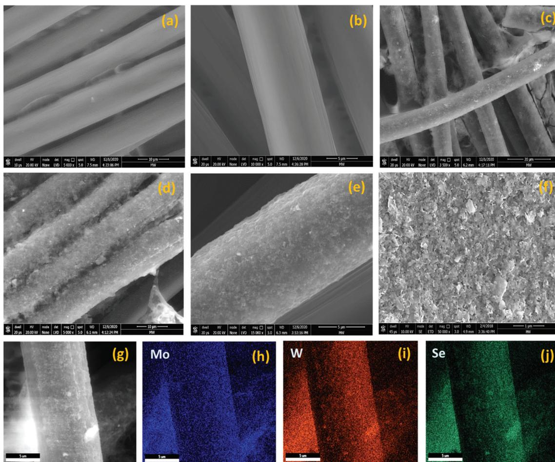
**Fig. 5** (a) The schematic illustration of MoSe<sub>2</sub>@WSe<sub>2</sub> HS film deposition on carbon fiber cloth by EPD. SEM images of (b and c) bare carbon fibers and (d and e) MoSe<sub>2</sub>@WSe<sub>2</sub> HS-coated carbon fibers. (f–j) EDAX elemental mapping of MoSe<sub>2</sub>@WSe<sub>2</sub> HS on single CF.
