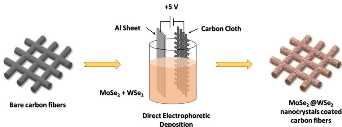
Fig. 1 Direct EPD of MoSe<sub>2</sub>@WSe<sub>2</sub> HS thin film on carbon cloth substrate.
