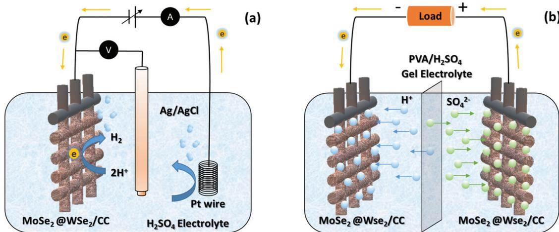
**Fig. 8** The schematic working mechanism of (a) hydrogen evolution and (b) FSSC-based on MoSe<sub>2</sub>@WSe<sub>2</sub> HS composite on CC.
