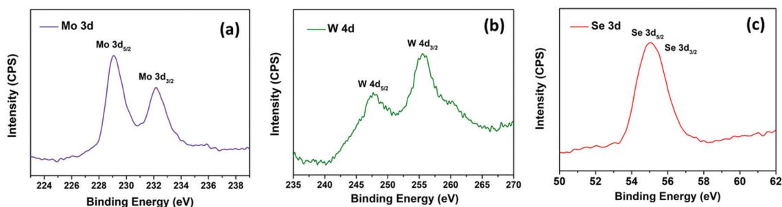
Fig. 4 XPS spectra of MoSe<sub>2</sub>@WSe<sub>2</sub>/CC (a) Mo 3d core level peaks region spectrum, (b) W 4d core level peaks region spectrum, (c) Se 3d core level peaks region spectrum.
