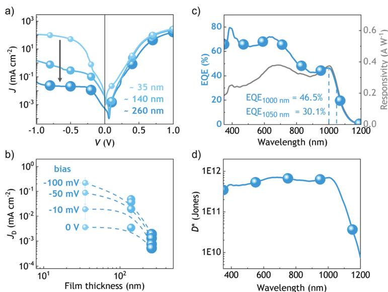
**Fig. 3** Photodetector performance of mixed AgBiS<sub>2</sub> devices. (a) Dark JV characteristics of devices using different AgBiS<sub>2</sub> layer thickness. (b) Dark current as a function of the photoactive layer thickness. The thickest device yielded the lowest dark current and best photodetector performance close to 0 V; (c) external quantum efficiency and responsivity spectra and (c) specific detectivity.
