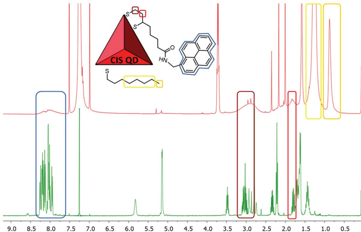
Fig. 3 <sup>1</sup>H-NMR (400 MHz, CDCl<sub>3</sub>) spectra of compound 1 (green line) and CIS@ZnS-py (red line), which is schematized in the inset. The principal signals are highlighted to show the broadening of the peaks related to the attached molecules.
