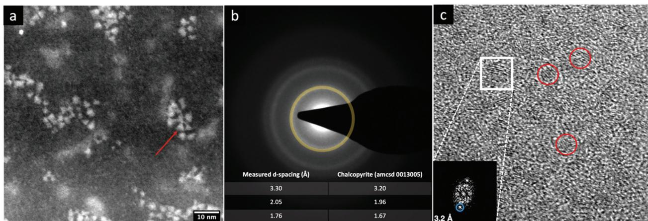
**Fig. 2** (a) High magnification STEM micrographs, selected area electron diffraction (SAED) and (c) high resolution (HR) TEM image of CIS@ZnS QDs. The FFT (fast Fourier transform) in the inset refers to the zone highlighted with the white square.
