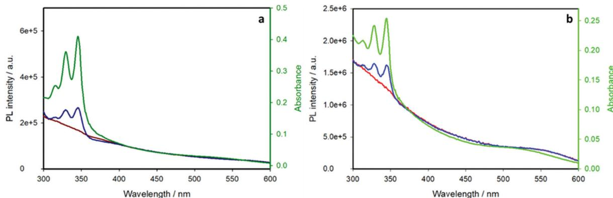
Fig. 7 Excitation spectra of (a) CIS QDs (dark red line) and CIS-py QDs (dark blue line) compared to the absorption spectrum of CIS-py QDs (green line) and (b) CIS@ZnS QDs (red line) and CIS@ZnS-py QDs (blue line) with the absorption profile of CIS@ZnS-py QDs in chloroform.  $\lambda_{em} = 700$  nm.
