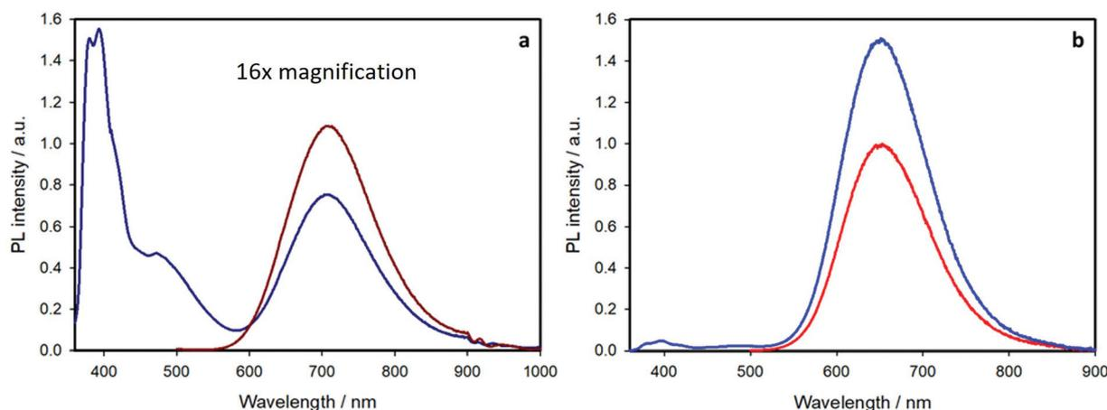
**Fig. 6** Emission spectra of equimolar suspensions of (a) CIS QDs (dark red line) and CIS-py QDs (dark blue line) and (b) CIS@ZnS QDs (red line) and CIS@ZnS-py QDs (blue line) in chloroform, exciting at 345 nm. The emission spectra in (a) are magnified by a 16 factor for comparison purposes.
