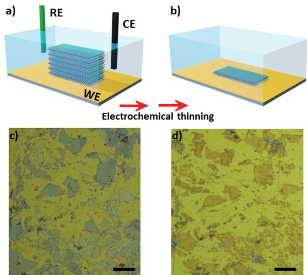
**Fig. 1** (a) Schematic view of the three-electrode cell. (b) Illustrative image of the electrode after electrochemical thinning process showing that bulk flakes are thinned down to monolayer. Optical microscope images of the electrodes containing MoS<sub>2</sub> flakes before (c) and after (d) electrochemical experiments. Scale bars are 100  $\mu\text{m}$ .
