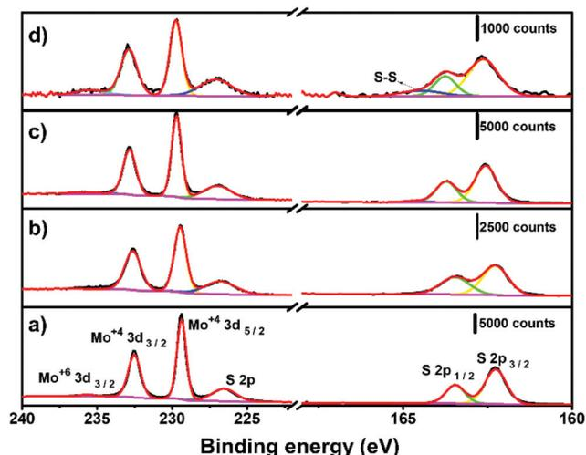
Fig. 5 XPS spectra for (a) bulk MoS<sub>2</sub> and at different electrochemical thinning times: (b) 5 s, (c) 20 s and (d) 240 s.
