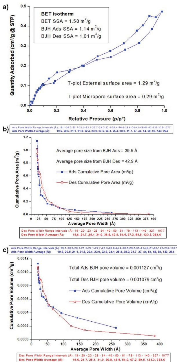
**Fig. 4** BET isotherm (a) and BJH cumulative pore area (b) and pore volume (c) plots for N<sub>2</sub> adsorption/desorption on sintered ceria scaffolds. The boxes show the pore width range intervals and pore width average data point values for adsorption (blue) and desorption (red).
