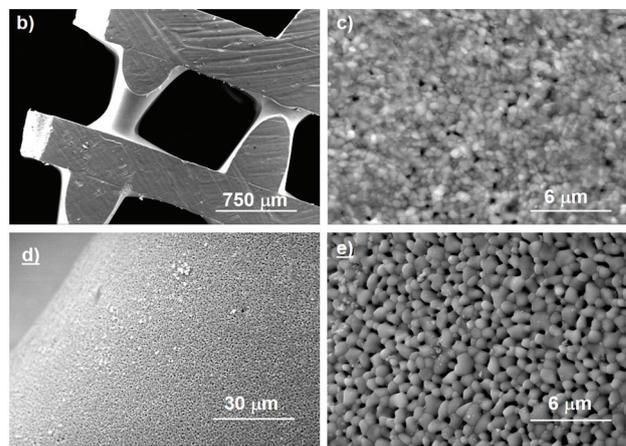
Fig. 3 XRD pattern of the ceria scaffold sintered at  $1450 \text{ °C}$ , with the major peaks for cubic  $\text{CeO}_2$  indexed. SEM images of a sintered and polished scaffold (b) show the interior (c) and exterior (d–e) microstructure.
