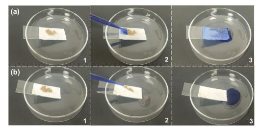
Fig. 7 The self-cleaning behavior of (a) pure cotton fabric and (b) SiO<sub>2</sub>-TiO<sub>2</sub>/PDMS coated superhydrophobic cotton fabric.
