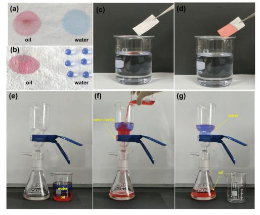
Fig. 8 Pictures of oil and water droplets on (a) the pure cotton fabric and (b) the SiO<sub>2</sub>-TiO<sub>2</sub>/PDMS-coated superhydrophobic cotton fabric. (c and d) Pictures of the absorbing process of n-hexane (dyed with Sudan IV) from water. (e-g) The dichloromethane-water mixture separation test of SiO<sub>2</sub>-TiO<sub>2</sub>/PDMS-coated superhydrophobic cotton fabric.
