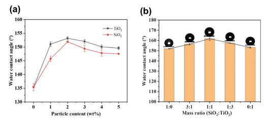
Fig. 3 (a) The WCA of the modified cotton fabric prepared from different contents of  $SiO_2$  and  $TiO_2$  particles when the content of PDMS was 2 wt%. (b) The WCA of the modified cotton fabric prepared from different mass ratios of the two particles.
