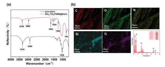
Fig. 1 (a) FTIR spectra of pure cotton fabric and SiO<sub>2</sub>-TiO<sub>2</sub>/PDMS-coated superhydrophobic cotton fabric. (b) Element distribution map and curve of SiO<sub>2</sub>-TiO<sub>2</sub>/PDMS-coated superhydrophobic cotton fabric.
