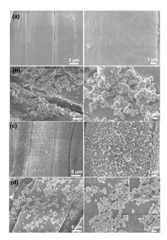
Fig. 2 SEM images of (a) pristine cotton fabric, (b) SiO<sub>2</sub>/PDMS-coated cotton fabric, (c)  $TiO_2/PDMS$ -coated cotton textile, and (d)  $SiO_2-TiO_2/PDMS$ -coated cotton textile cotton PDMS-coated cotton fabric
