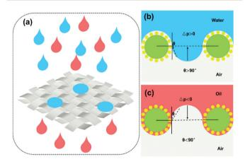
Fig. 10 (a) Schematic diagram of oil-water separation on SiO<sub>2</sub>-TiO<sub>2</sub>/ PDMS-coated superhydrophobic cotton fabric. (b) Superhydrophobic cotton fabric can block water due to  $\Delta p > 0$ . (c) Superhydrophobic cotton fabric can absorb oil due to  $\Delta p < 0$ .
