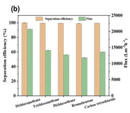
Fig. 9 (a) Separation efficiency and flux of a dichloromethane/water mixture during separation cycles. (b) Separation efficiency and flux for separating various immiscible oil/water mixtures.
