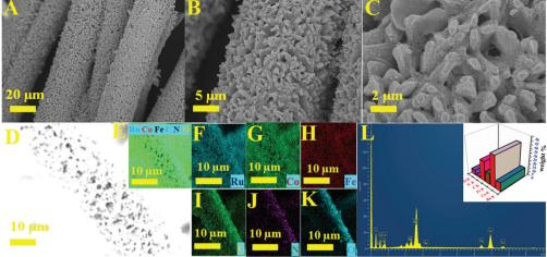
Fig. 2 (A-C) Low and high magnification FESEM images of Ru MOF CoFe nanoarrays. (D) Electron image and (E) elemental mapping images of Ru (F), Co (G), Fe (H), C (I), N (J), and O (K). (L) EDX spectrum and inset image corresponding to elemental composition images of Ru MOF CoFe nanoarrays.
