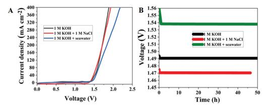
Fig. 9 (A) LSV curves of Ru MOF CoFe nanoarray performance in artificial seawater and natural seawater electrolysis. (B) Long-term stability measurements of Ru MOF CoFe nanoarrays performed at a constant current cell voltage in different electrolytes.
