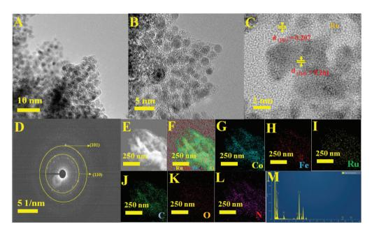
Fig. 3 (A and B) Different magnification TEM images. (C) High-resolution TEM image with lattice fringe. (D) SAED patterns. (E) STEM image. (F) The corresponding TEM elemental maps of (G) Co, (H) Fe, (I) Ru, (J) C, (K) O and (L) N elements. (M) TEM EDX spectrum of Ru MOF FeCo nanoarrays.
