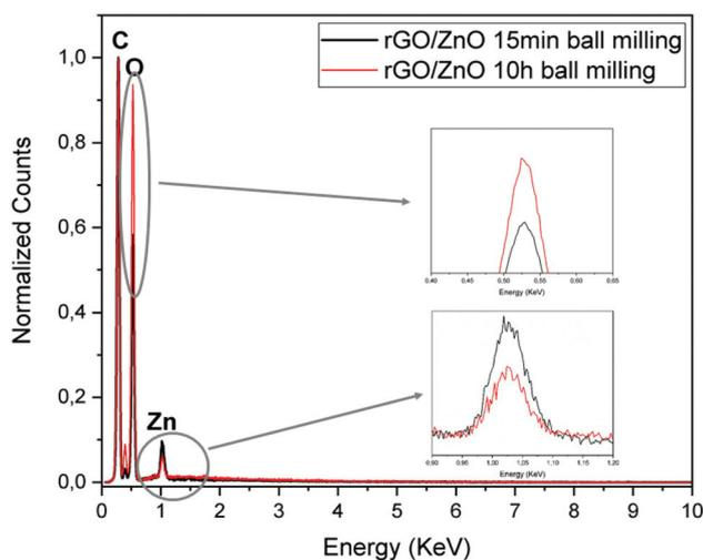
Fig. 5 EDX results of the rGO/ZnO hybrid composite.
