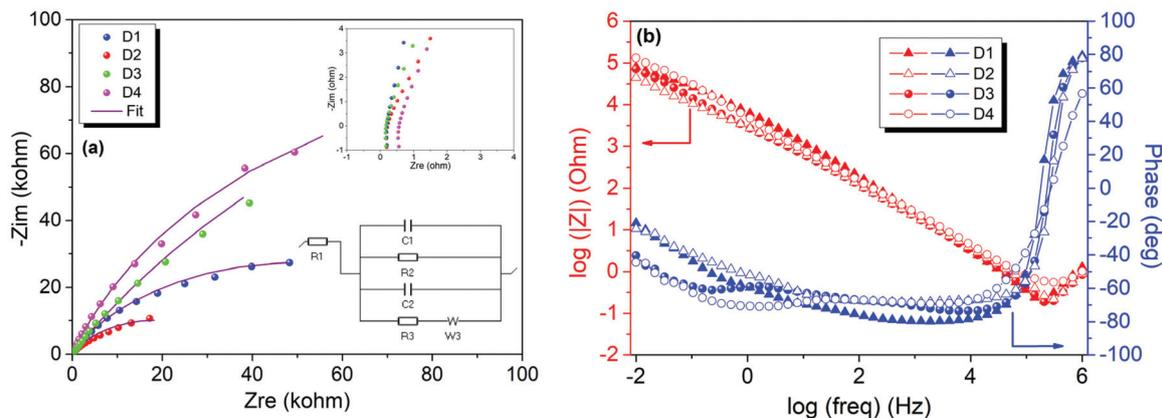
**Fig. 8** Electrochemical impedance spectra of the asymmetric supercapacitors D1, D2, D3 and D4 with a 6 M KOH electrolyte. (a) Nyquist plot (top inset: high frequency region and bottom inset: equivalent circuit used to fit the experimental data) and (b) Bode plot.
