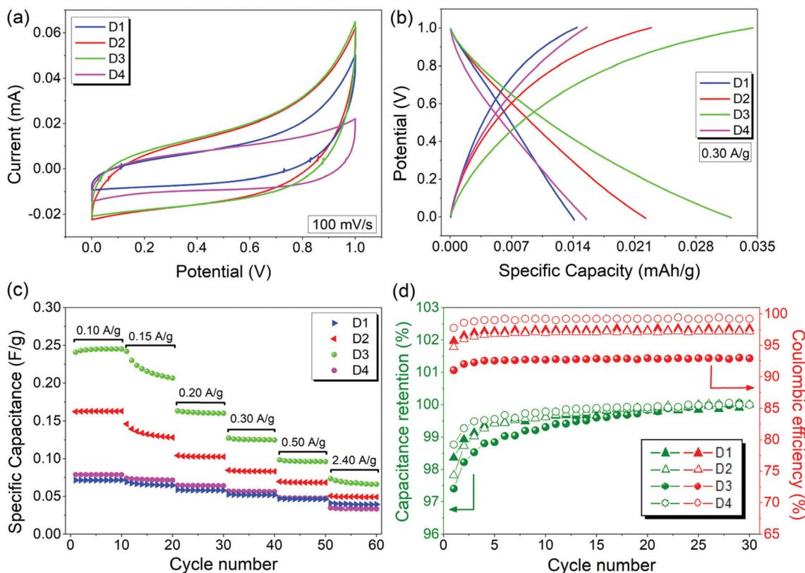
Fig. 9 Electrochemical performances of supercapacitors D1, D2, D3 and D4 with a 6 M KOH electrolyte: (a) CV taken at a 100 mV s<sup>-1</sup> scan rate, (b) charge–discharge curves cycled between 0 and 1 V at a current density of 0.30 A g<sup>-1</sup>, (c) specific capacitances at various current densities, and (d) comparison of the capacitance retention of D1, D2, D3 and D4.
