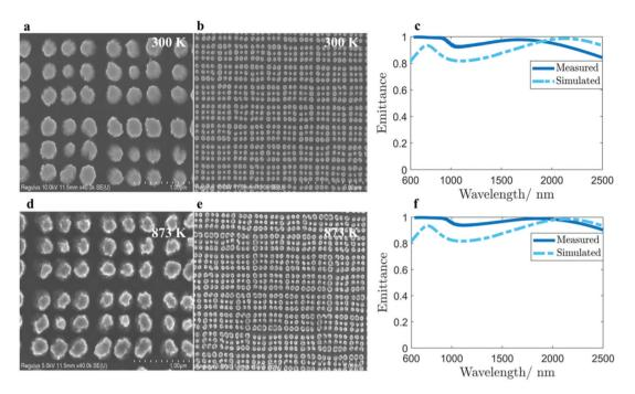
Fig. 5 SEM images of the emitter and the measured emittance (a) at 300 K with a scale bar of 1  $\mu$ m and (b) at 300 K with a scale bar of 5  $\mu$ m. (c) Comparison of the measured and simulated emittances at 300 K, (d) at 873 K with a scale bar of 1  $\mu$ m, and (e) at 873 K with a scale bar of 5  $\mu$ m. (f) Comparison of the measured and simulated emittances at 873 K.
