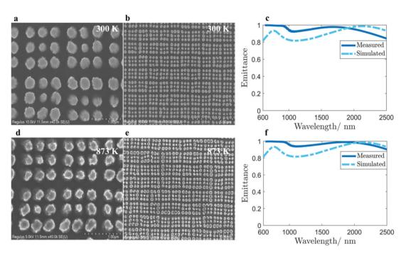
Fig. 5 SEM images of the emitter and the measured emittance (a) at 300 K with a scale bar of 1  $\mu$ m and (b) at 300 K with a scale bar of 5  $\mu$ m. (c) Comparison of the measured and simulated emittances at 300 K, (d) at 873 K with a scale bar of 1  $\mu$ m, and (e) at 873 K with a scale bar of 5  $\mu$ m. (f) Comparison of the measured and simulated emittances at 873 K.
