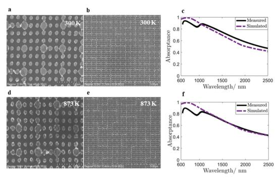
Fig. 3 SEM images of the absorber and the measured absorptance (a) at 300 K with a scale bar of 1 µm and (b) at 300 K with a scale bar of 5 µm. (c) Comparison of the measured and simulated emittances at 300 K, (d) at 873 K with a scale bar of 1 µm, and (e) at 873 K with a scale bar of 5 µm. (f) Comparison of the measured and simulated emittances at 873 K.
