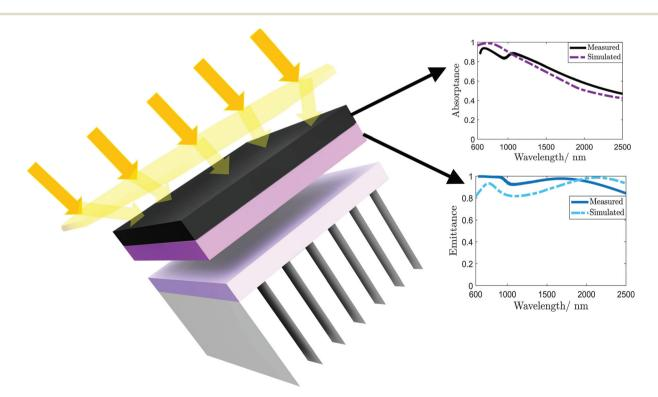
Fig. 1 Theoretical concept of STPVs with actual results from the proposed absorber/emitter designs. This figure is not made up to the proportion.
