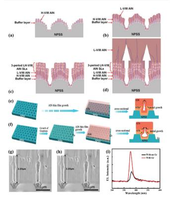
Fig. 6 (a-d) Schematic illustrations of growth evolution for AlN epilayers on NPSS. Reproduced with permission. 110 Copyright 2018, Elsevier. Schematic diagrams of AlN growth on (e) bare NPSS and (f) Gr/ NPSS. Cross-sectional schematic diagrams of AlN films grown on (g) bare NPSS and (h) Gr/NPSS. (i) EL spectra of the DUV-LEDs with and without the graphene interlayer. Reproduced with permission. 116 Copyright 2019, American Institute of Physics Publishing.
