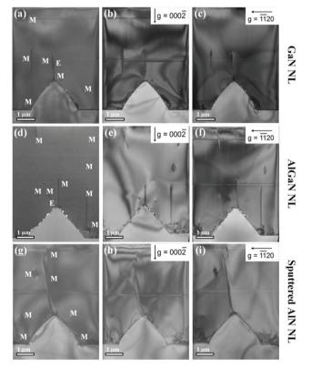
Fig. 4 Cross-sectional TEM images of UV LEDs grown on (a-c) LT-GaN NL/PSS, (d-f) LT-AlGaN NL/PSS and (g-f) sputtered AlN NL/PSS. The edge (E) and mixed (M) type dislocations are marked. Reproduced with permission. 107 Copyright 2017, Springer Nature Publishing Group.
