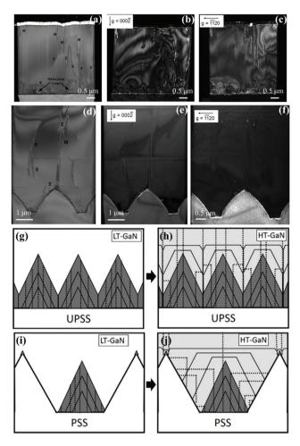
Fig. 3 TEM images of GaN epitaxial layer grown on (a-c) FSS and (d-f) PSS. Reproduced with permission.<sup>56</sup> Copyright 2015, Elsevier. Formation and propagation mechanism of dislocation with (g-h) FSS and (i-j) PSS. Reproduced with permission.<sup>99</sup> Copyright 2018, Elsevier.
