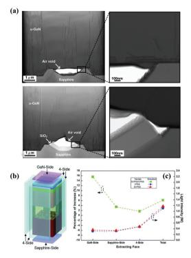
Fig. 11 (a) TEM images of LEDs grown on volcano-shaped PSS (VPSS) and volcano-shaped PSS with embedded SiO<sub>2</sub> (SVPSS). (b) Schematic of different receiver positions in the simulation. (c) Light intensity and percentage increase in light intensity of LEDs grown on the VPSS and SVPSS. Reproduced with permission. 142 Copyright 2015, Royal Society of Chemistry.
