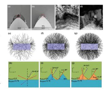
Fig. 15 Cross-sectional STEM images of AlGaN grown (a) on PSS and (b) PSSA. (c) Enlarged STEM images of the marked areas in (a) and (d) that in (b). Cross-sectional ray-tracing images of top-emitting UV LEDs on (e) FSS, (f) PSS, and (g) PSSA. Schematic illustration of light trajectories in top-emitting UV LEDs on (h) FSS, (i) PSS, and (j) PSSA. Reproduced with permission.<sup>24</sup> Copyright 2019, Elsevier.
