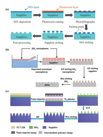
Fig. 2 (a) The fabrication process flow for PSS. (b) The fabrication process flow for NPSS by self-assembled SiO<sub>2</sub> nanosphere monolayer template. Reproduced with permission.<sup>44</sup> Copyright 2014, American Institute of Physics Publishing. (c) The fabrication process flow for NPSS by nanoimprint lithography. Reproduced with permission.<sup>45</sup> Copyright 2016, Springer Nature Publishing Group.
