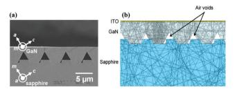
Fig. 14 (a) Cross-sectional SEM images of (11–22) GaN layer on r-plane PSS. (b) Ray tracing result of (11-22) LED structure on r-plane PSS with embedded air voids. Reproduced with permission. 170 Copyright 2011, John Wiley and Sons.
