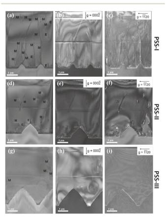
Fig. 5 Cross-sectional TEM images of UV LEDs grown on (a-c) PSS I, (d-f) PSS II and (q-i) PSS III. The screw (S), edge (E), and mixed (M) type dislocations are marked. Reproduced with permission. 108 Copyright 2017, Institute of Physics.
