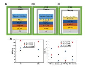
Fig. 9 Simulation model of (a) flip-chip DUV LED on FSS (DUV LED-I), (b) flip-chip DUV LED on NPSS (DUV LED-II), and (c) flip-chip DUV LED with roughed n-AlGaN surface (DUV LED-III). (d) Simulated LEE of DUV LED-I, DUV LED-II, and DUV LED-III. Reproduced with permission. Copyright 2020, Institute of Physics.
