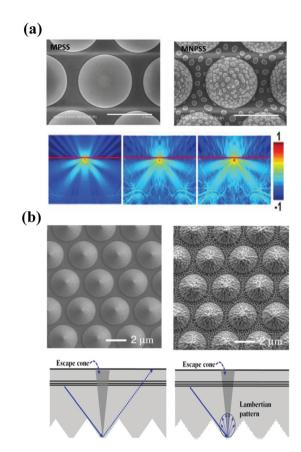
**Fig. 17** (a) Top-view SEM images of MPSS and NMCPSS and cross-sectional FDTD simulation images of light intensity distribution of FSS, MPSS- and NMCPSS-based LEDs. Reproduced with permission.<sup>178</sup> Copyright 2013, Institute of Physics. (b) Top-view SEM images and light tracing schematic diagrams of MPSS and NMCPSS. Reproduced with permission.<sup>179</sup> Copyright 2016, American Chemical Society.
