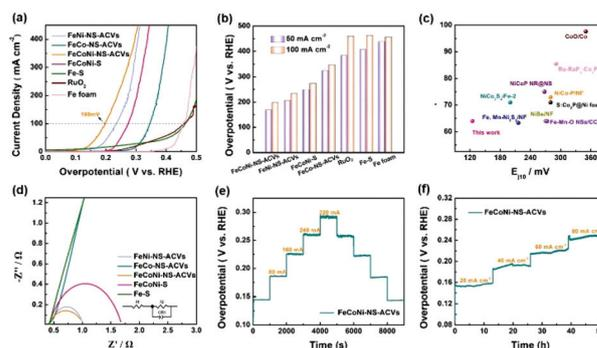
**Fig. 3** Electrochemical measurements: (a) OER polarization curves, (b) overpotential comparison at  $50\text{ mA cm}^{-2}$  and  $100\text{ mA cm}^{-2}$ , (c) comparison of the overpotentials ( $E_{j10}$ ) and Tafel slopes with the references, (d) Nyquist plots, and (e and f) stability tests of the obtained catalysts in 1 M KOH.
