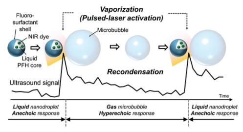
Fig. 8 Vaporisation and recondensation of laser-activated nanodroplets. When activated, nanodroplets immediately produce strong ultrasound signals<sup>107</sup> (this figure has been reproduced from ref. 107 with permission from John Wiley and Sons, copyright 2017).
