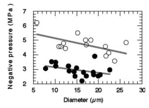
Fig. 4 Relationship between the pressure threshold for ADV and diameter of nanodroplets. Decreasing the droplet diameter will increase pressures for vaporisation<sup>73</sup> (this figure has been reproduced from ref. 73 with permission from Royal Society of Chemistry, copyright 2004).
