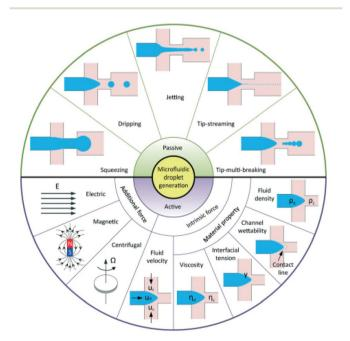
**Fig. 6** Schematic of droplet generation in passive and active methods<sup>95</sup> (this figure has been reproduced from ref. 95 with permission from Royal Society of Chemistry, copyright 2001).
