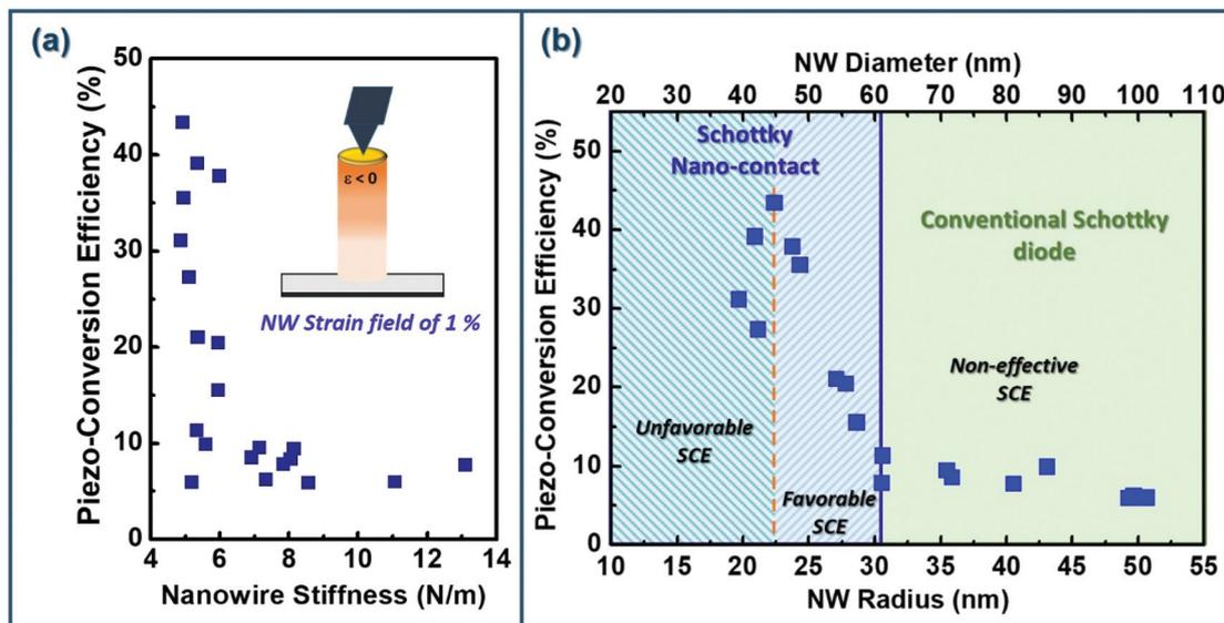
**Fig. 6** (a) Electromechanical coupling coefficient,  $\eta$ , variation as a function of the NW stiffness for a deformation of 1%. The variation in the 5.9–43.4% range highlights that the coupling coefficient is not only driven by the NW mechanical characteristics. (b) Variation of  $\eta$  as a function of the NW radius. The OV can also be affected both by the behaviour of the Schottky diode harvesting the generated OV, and by the influence of the surface charge effects (SCE).
