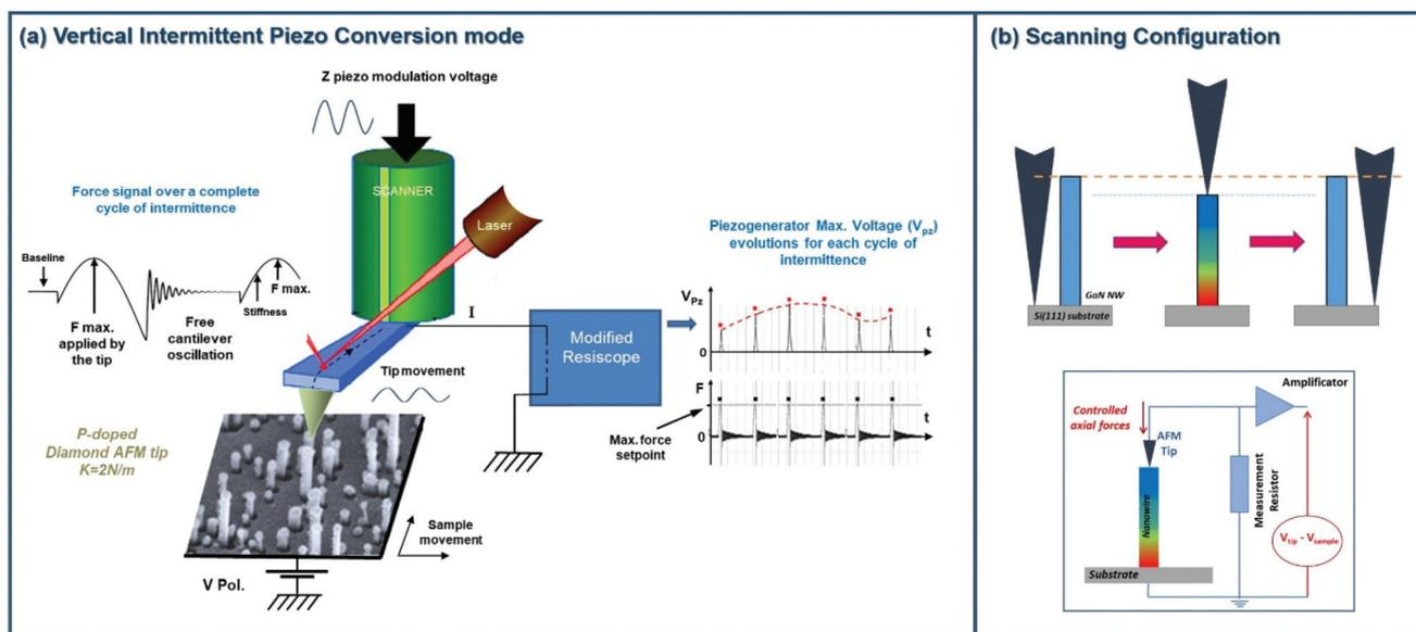
**Fig. 1** (a) Schematic view of the new conducting AFM technique working in intermittent-contact piezoelectric mode, inspired by the so-called 'pulsed force mode' (PFM). Combined with a specifically adapted Resiscope module, the AFM system allows quantifying the piezoelectric response of individual GaN NWs resulting from their deformation under a well-controlled axial normal force; (b) schematic views of the measurement principle and of the equivalent electrical circuit of the AFM system.
