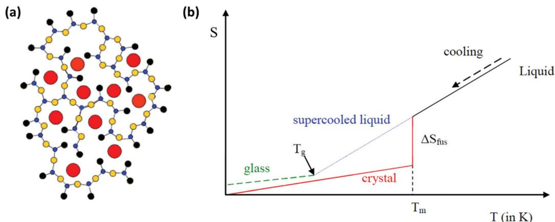
**Fig. 1** (a) Schematic representation of the sodium silicate glass network in two dimensions. Red circles represent sodium cations, blue circles represent silicon atoms, yellow circles represent bridging oxygen atoms, and black circles represent non-bridging oxygen atoms (a has been adapted from ref. 4 with permission from John Wiley and Sons, copyright 2006). (b) Entropy variation versus temperature when a liquid is cooled towards absolute zero.
