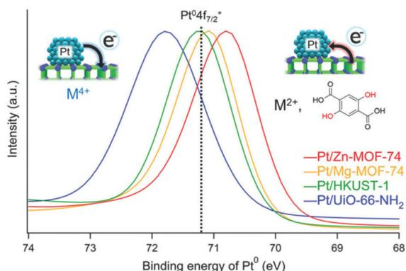
Fig. 8 Fitted curves (Pt<sup>0</sup> 4f<sub>7/2</sub>) of XPS spectra of (red) Pt/Zn-MOF-74, (yellow) Pt/Mg-MOF-74, (green) Pt/HKUST-1, and (blue) Pt/UiO-66-NH<sub>2</sub>. The black dotted line indicates the binding energy of bulk Pt<sup>0</sup> 4f<sub>7/2</sub>.
