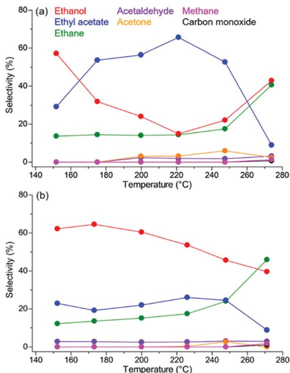
Fig. 13 Selectivity for each product on (a) Pt/Uio-66-NH<sub>2</sub> and (b) Pt/MIL-125-NH<sub>2</sub>. This figure has been reproduced from ref. 45 with permission from the American Chemical Society, copyright 2021.
