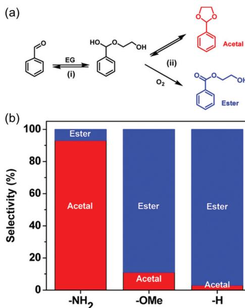
Fig. 7 (a) Scheme of the aerobic reaction between benzaldehyde and ethylene glycol (EG). (b) Product selectivity on Pd@UiO-66-X (X = NH<sub>2</sub>, OMe, and H). This figure has been reproduced from ref. 41 with permission from the American Chemical Society, copyright 2016.
