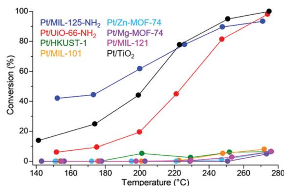
Fig. 12 Conversion of AcOH on Pt/MOFs and Pt/TiO<sub>2</sub>. This figure has been reproduced from ref. 45 with permission from the American Chemical Society, copyright 2021.
