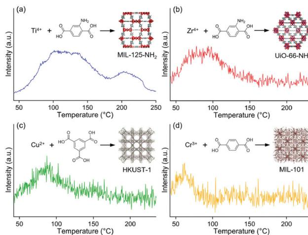
Fig. 11 TPD-MS charts of (a) MIL-125-NH<sub>2</sub>, (b) UiO-66-NH<sub>2</sub>, (c) HKUST-1, and (d) MIL-101 at *m/z* = 60 (for AcOH molecule). This figure has been reproduced from ref. 45 with permission from the American Chemical Society, copyright 2021.
