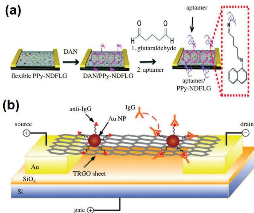
**Fig. 10** (a) Illustration of N-doped graphene FET biosensor for detection of VEGF, reproduced from ref. 135 with permission from [Wiley-VCH], copyright [2012], (b) graphene FET schematic for detection of protein high binding occurrences, reproduced from ref. 136 with permission from [Wiley-VCH], copyright [2010].
