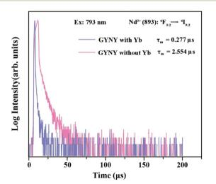
Fig. 4 Luminescence decay curves of  $Nd^{3+}$  emissions measured at 893 nm for GYNY with and without  $Yb^{3+}$  nanocrystals by pulsed 793 nm excitation.
