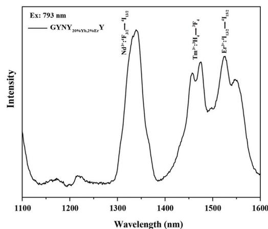
**Fig. 2** Downshifting emission spectrum of  $\text{NaGdF}_4:49\%\text{Yb},1\%\text{Tm}@/\text{NaYF}_4:20\%\text{Yb}@/\text{NaNdF}_4:10\%\text{Yb}@/\text{NaYF}_4:20\%\text{Yb},2\%\text{Er}@/\text{NaYF}_4$  nanocrystals.
