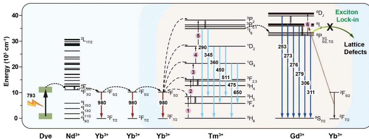
Fig. 6 Schematic energy diagram of the cascade energy transfer within a dye-sensitized heterogeneously doped-lanthanide nanocrystal.
