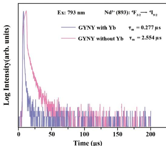
Fig. 4 Luminescence decay curves of Nd<sup>3+</sup> emissions measured at 893 nm for GYNY with and without Yb<sup>3+</sup> nanocrystals by pulsed 793 nm excitation.
