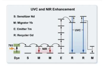
Scheme 1 Schematic illustration of the dye-sensitized upconversion and downshifting mechanism for UVC and NIR generation.
