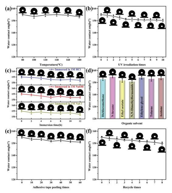
Fig. 6 Variations in the WCA of the PEI/TMSPA/SiO<sub>2</sub>/DTMS fabric after (a) heating at different temperatures for 2 h, (b) UV irradiation with different times, (c) treatment in 1 M NaCl, HCl, and NaOH solutions for different times, (d) immersion in different organic solvents for 24 h, (e) adhesive tape peeling test and (f) washing test.
