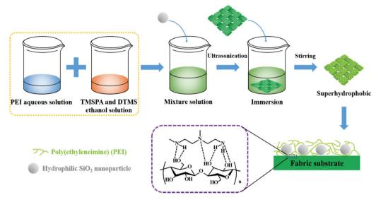
Scheme 1 Schematic of fabrication of superhydrophobic PEI/TMSPA/SiO<sub>2</sub>/DTMS fabrics.
