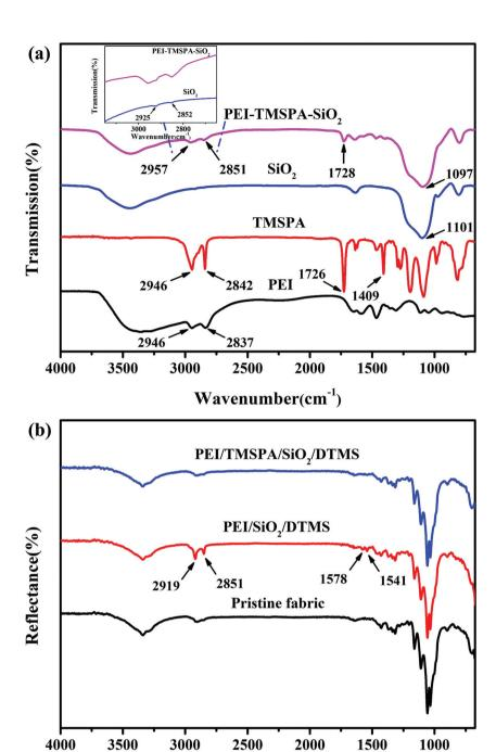
Fig. 2 FTIR spectra of (a) PEI-TMSPA-SiO<sub>2</sub>, pure SiO<sub>2</sub>, TMSPA and PEI, and (b) pristine fabric, PEI/SiO<sub>2</sub>/DTMS fabric and PEI/TMSPA/SiO<sub>2</sub>/DTMS fabric
