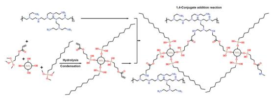
Fig. 4 Schematic illustration of a mechanism of superhydrophobic fabric during the fabrication process.
