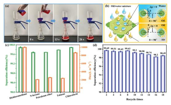
Fig. 7 (a) Schematic of oil/water separation using PEI/TMSPA/SiO<sub>2</sub>/DTMS fabrics. (b) Schematic of oil/water mixture separation mechanism of coated fabrics. (c) Separation efficiencies and fluxes of different oil/water mixtures. (d) The separation efficiency of the dichloromethane/water mixture after multiple separation cycles.
