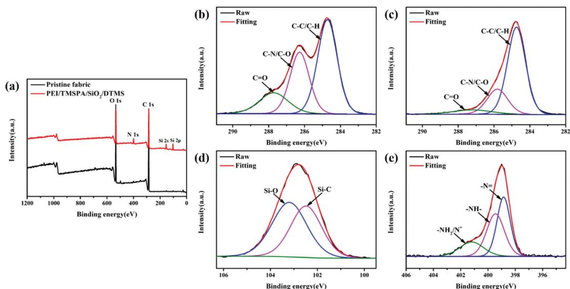
Fig. 3 (a) XPS spectra of pristine and PEI/TMSPA/SiO<sub>2</sub>/DTMS fabrics. C 1s XPS spectra with fitting curves of (b) pristine and (c) PEI/TMSPA/SiO<sub>2</sub>/DTMS fabrics. (d) Si 2p XPS spectra and (e) N 1s XPS spectra with fitting curves of the PEI/TMSPA/SiO<sub>2</sub>/DTMS fabric.
