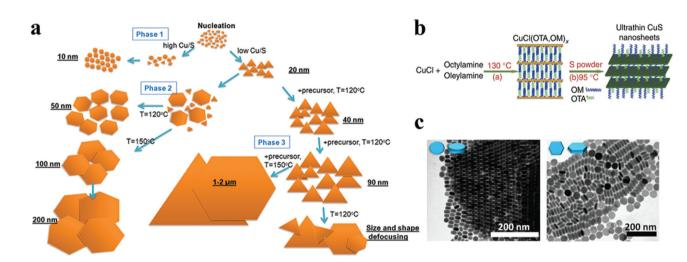
Fig. 4 (a) The shape transformations during the OAm–S based hot-injection copper sulphide synthesis are shown in a scheme, along with methods to control the shape. Reproduced from ref. 115 with permission from RSC, copyright 2018; (b) schematic illustration of fabrication of ultrathin CuS nanosheets.  $^{74}$  ©2012 Nature (c) TEM images showing the morphology evolution of  $Cu_{2-x}S$  NCs. Reproduced from ref. 118 with permission from RSC, copyright 2011 ©2011 RSC.
