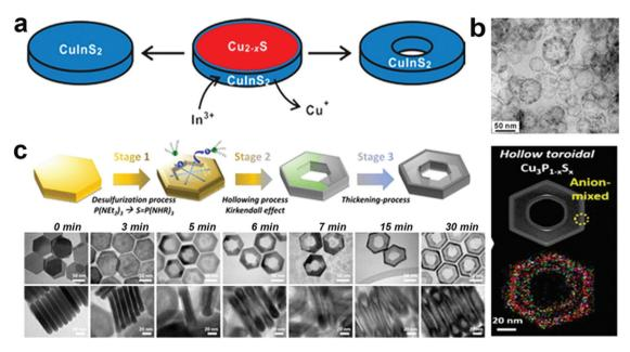
Fig. 3 (a) Illustration of the nanoscale Kirkendall mechanism on the  $Cu_{2-x}S$  template for forming (b) hollow  $CuInS_2$  nanoplates; reproduced from ref. 110 with permission from ACS, copyright 2015; (c) schematics and low resolution TEM of  $Cu_3P_{1-x}S_x$  toroidal ring formation mechanism. The STEM-EDS elemental mapping displays the homogeneous signal of Cu (red), P (green) and S (blue) on the toroidal ring. Reproduced from ref. 64 with permission from ACS, copyright 2020.
