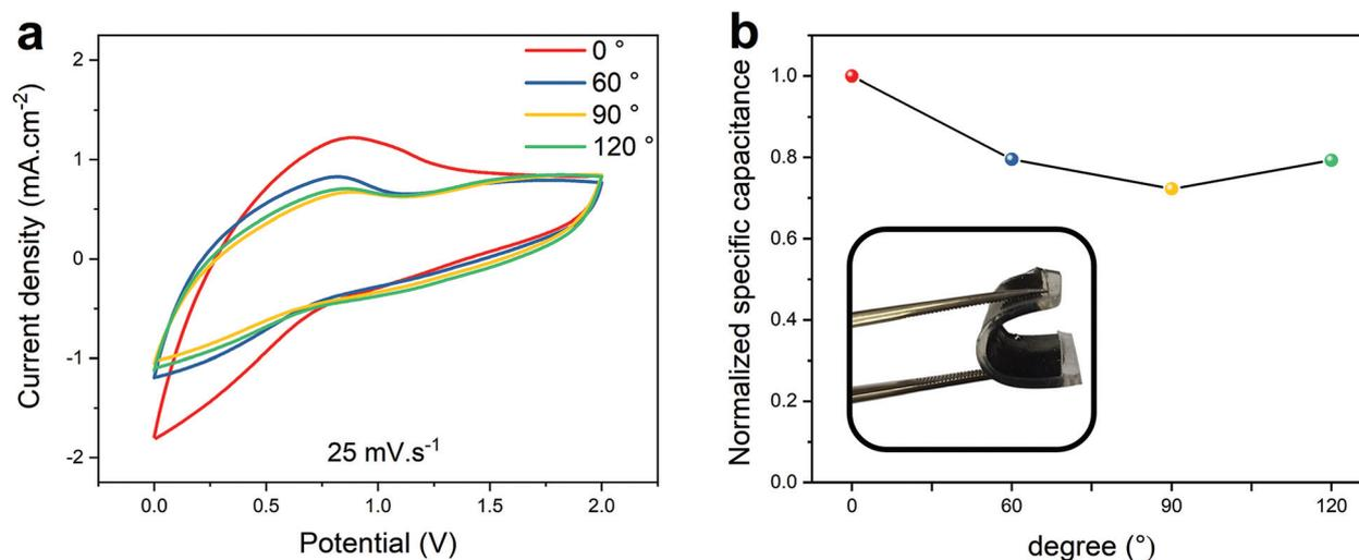
**Fig. 8** Performance of the ACNTA-PANI/PDMS device under different bending angles. (a) CV curves at 25 mV s<sup>-1</sup>. (b) Normalized specific capacitance calculated from the CV curves over the bent angle. The inset illustrates the flexibility of the devices under different angles.
