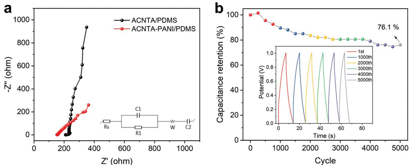
**Fig. 6** Electrochemical performance of symmetric two-electrode supercapacitors. (a) EIS curve of ACNTA-PANI/PDMS at frequencies varying between  $10^{-1}$  and  $10^5$  Hz; the inset shows the equivalent circuit used for fitting the experimental data. (b) GCD stability of ACNTA-PANI/PDMS in a potential range between 0 and 1 V for 5000 cycles.
