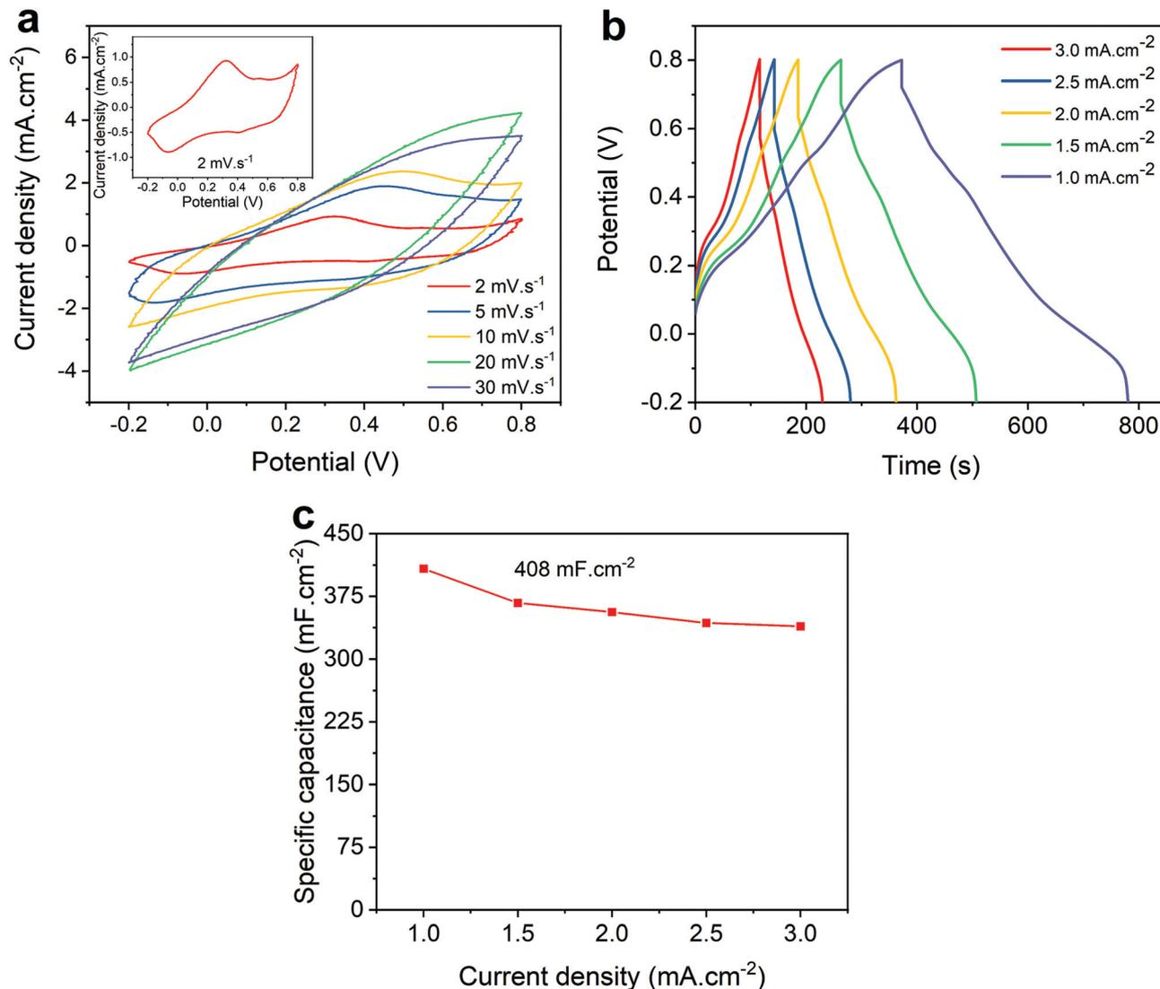
Fig. 4 Electrochemical performance of ACNTA-PANI/PDMS measured in a three-electrode configuration. (a) CV curves of the electrodes at different scan rates from 2 to 30 mV s<sup>-1</sup>. The inset shows the CV curve at a scan rate of 2 mV s<sup>-1</sup>. (b) GCD curves at different current densities varying from 1 to 3 mA cm<sup>-2</sup>. (c) Areal specific capacitance calculated from GCD curves.
