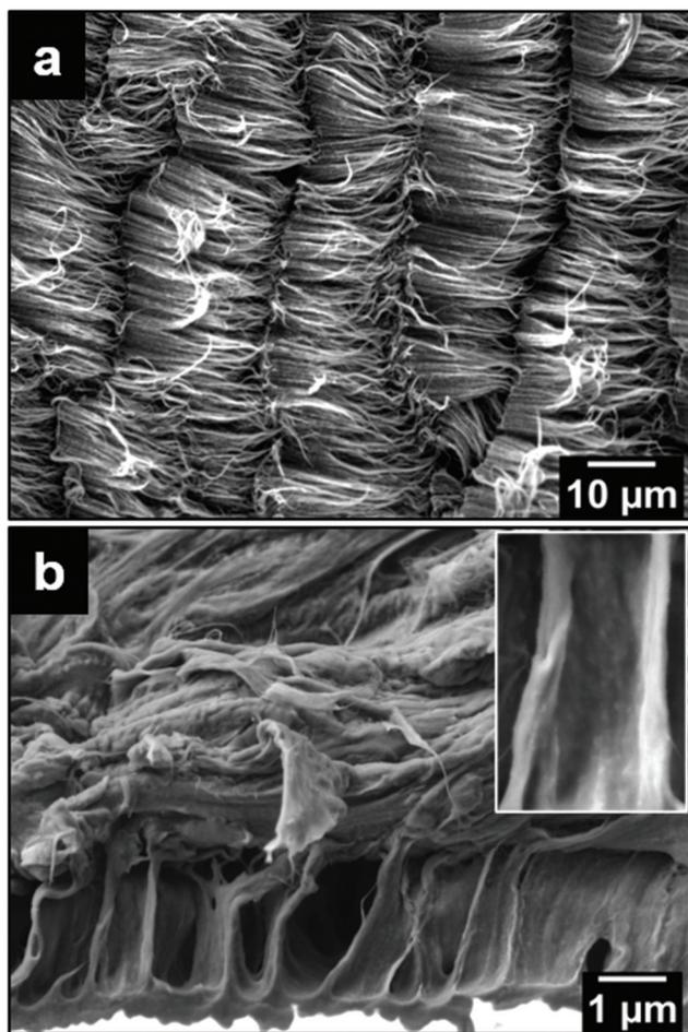
**Fig. 2** (a) Top-view SEM image of the horizontally aligned carbon nanotubes (HA-CNTs) that were bent during the wafer drop casting process. (b) Cross-sectional SEM image of the flexible electrode showing HA-CNTs on top of vertically aligned carbon nanotubes (VA-CNTs) densified when in contact with the polydimethylsiloxane (PDMS) matrix. PANI is a thin indistinguishable layer spread across the HA-CNTs/air interface.
