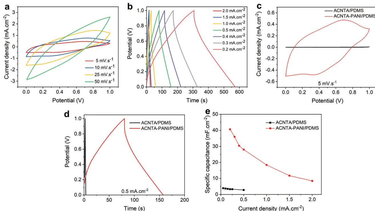
**Fig. 5** Electrochemical performance of symmetric two-electrode supercapacitors. (a) CV curves of ACNTA-PANI/PDMS at scan rates varying between 5 and 50  $\text{mV s}^{-1}$ . (b) GCD curves at different current densities. (c) CV curves of ACNTA/PDMS and ACNTA-PANI/PDMS at a scan rate of 5  $\text{mV s}^{-1}$ . (d) GCD curves of ACNTA/PDMS and ACNTA-PANI/PDMS at 0.5  $\text{mA cm}^{-2}$ . (e) Areal specific capacitances calculated for different current densities.
