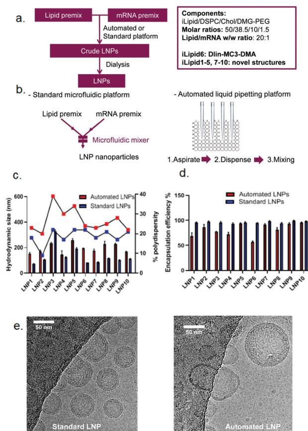
**Fig. 4** LNP preparation platforms and characterisation of ten novel LNPs-mRNA. (a) Formulation fabrication scheme (left) and components (right) of LNPs. (b) Key steps to fabricate mRNA LNPs using standard (left) and automated (right) platforms. Hydrodynamic size and PDI (c), mRNA encapsulation efficiency (d) and representative cryoTEM images (e) of the resulting mRNA LNPs fabricated with standard and automated platform.
