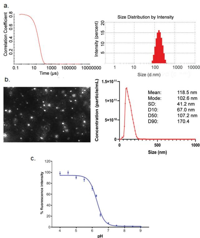
**Fig. 2** Physicochemical characterisation of mRNA MC3-LNPs produced with the automated platform. (a) Correlogram (left) of dynamic light scattering (DLS) measurements and size distribution of nanoparticles (right). (b) Visualized nanoparticle tracking (left) and size distribution from nanoparticle tracking analysis (NTA, right). (c) TNS assay of the automated LNPs.
