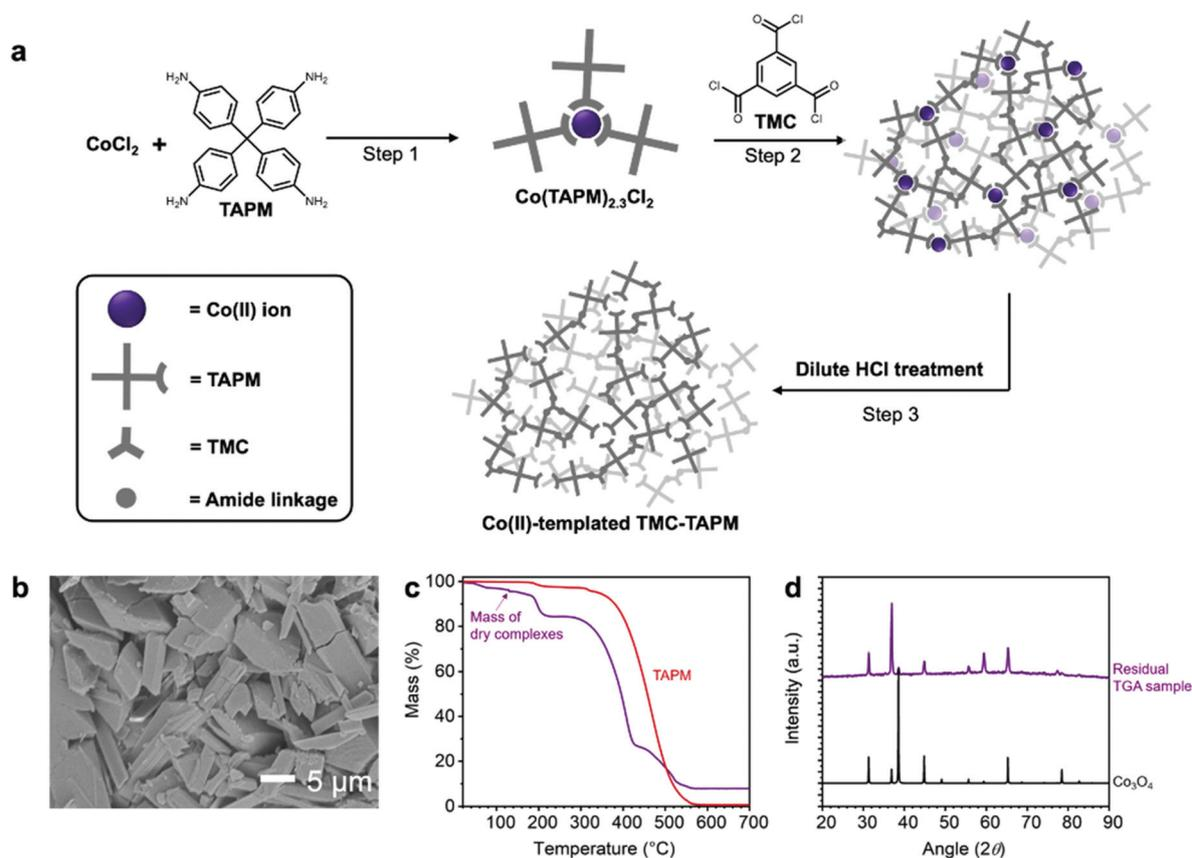
**Fig. 2** (a) Schematic representation of the synthesis of  $\text{Co(II)}$ -templated TMC-TAPM. (b) Scanning electron microscope image of  $\text{Co(TAPM)}_{2.3}\text{Cl}_2$  complexes. (c) Thermogravimetric analysis of  $\text{Co(TAPM)}_{2.3}\text{Cl}_2$  complexes (purple) and TAPM (red). (d) Powder X-ray diffraction spectra of residual TGA sample (purple) and  $\text{Co}_3\text{O}_4$  (black).
