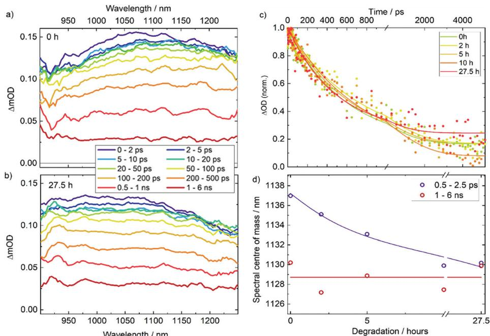
**Fig. 3** Transient absorption spectra for neat  $\text{AgBiS}_2$  films after (a) 0 h and (b) 27.5 h degradation following a 700 nm excitation. (c) Evolution in time of the normalised TA PIA signal for all films. (d) Centre of mass of PIA signal as a function of degradation time for early and late pump–probe time delays.
