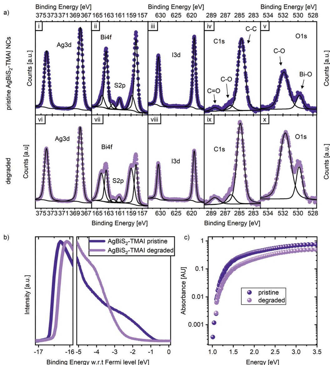
**Fig. 5** The degradation of AgBiS<sub>2</sub>-TMAI NCs. (a) XPS data of a pristine film in the top row, bottom row presents the state after 24 h of dry air and sunlight exposure. The scale is arbitrary but the same for each orbital. (b) UPS data for a pristine and 17 h degraded AgBiS<sub>2</sub>-TMAI film on ITO. (c) PDS measurement of the absorption of a pristine and 24 h degraded film.
