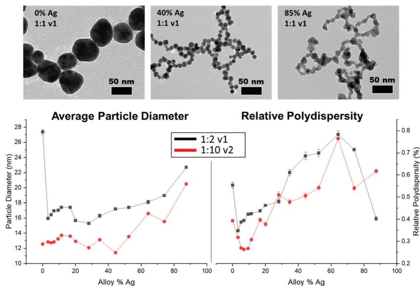
**Fig. 3** TEM images (top) show that NPs display increasing polydispersity and significant instability as a function of increased Ag content, which was observed regardless of reduction conditions utilized. Representative SAXS results (bottom) display statistical trends in NP size and polydispersity, reported as the actual Ag% in the NP (as determined by XRF). Consistently, larger reductant ratios result in smaller, more uniform NPs.
