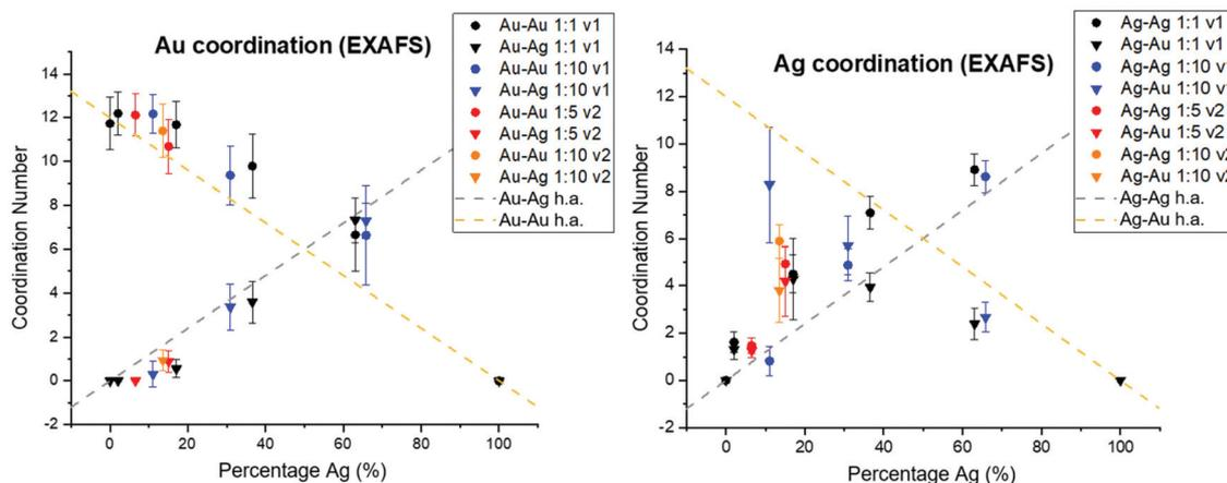
**Fig. 6** Au (left) and Ag (right) coordination numbers derived from EXAFS fitting show deviation from homogeneity as a function of solution Ag percentage (%), compared with the theoretically expected trends (designated as h.a. for homogeneous alloy) plotted in dashed lines. Au–Au bonding consistently dominates over Au–Ag, and Ag–Ag bonding over Ag–Au.
