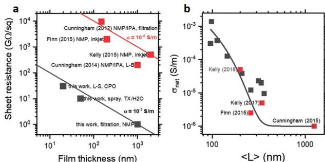
**Fig. 3** (a) Sheet resistance vs film thickness showing thinner films and higher conductivities for Langmuir films and other MoS<sub>2</sub> networks in this work compared to literature values. (b) Conductivity vs average nanosheet length showing exponent decay with length, for both size-selected few-layer networks and larger thicker nanosheets reported in literature.
