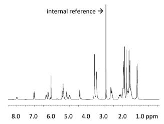
Fig. 7  $\,^{1}$ H NMR spectrum (300 MHz) of COR A produced by the strain Corallococcus coralloides B035 (COR A batch – content 99%) in acetonitrile-d<sub>3</sub>/D<sub>2</sub>O (6:1) with the internal reference dimethyl sulfone.<sup>54</sup>
