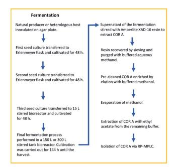
Fig. 6 Fermentation and downstream process for COR A, resulting in a recovery rate of >80%. RP-MPLC (reversed-phase medium pressure liquid chromatography).<sup>54</sup>
