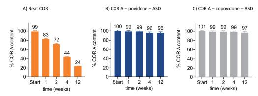
Fig. 12 Increased stability of the COR A-ASD formulations compared to neat COR A when stored in closed twist-off glass vials under nitrogen at 30 °C/65% RH, determined via HPLC-DAD (COR A batch – content 99%).<sup>54</sup>
