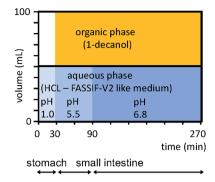
Fig. 9 Biphasic dissolution media setup and profiles of the neat COR A performed under simulated fasted human gut conditions (n = 3, 100% $\hat{=}~0.2~{
