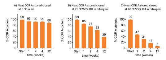
Fig. 10 Stability analysis at 5, 25 and 40 °C via HPLC-DAD of neat COR A in closed twist-off glass vials (gas tight) and two different gas environments within the vials (air or nitrogen, n = 3, mean, SD, COR A batch – content 99%, RH = relative humidity).<sup>53,54</sup>
