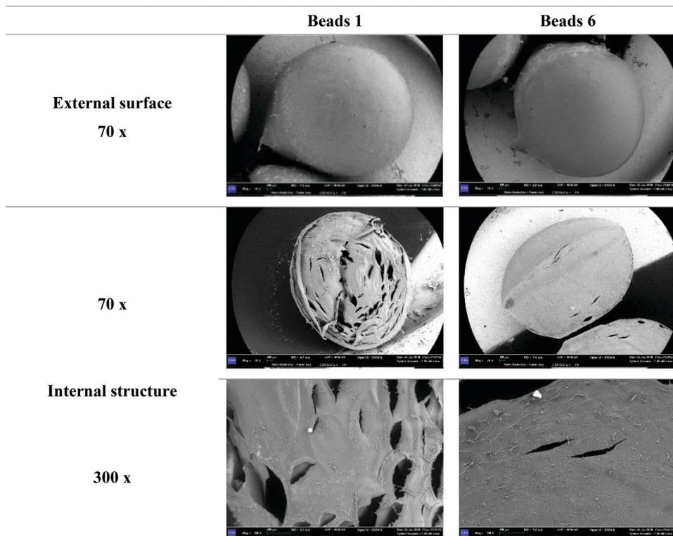
Fig. 5 SEM images at 70x magnification of the external structure and at 70x and 300x magnifications of the internal structure of **Beads 1** and **Beads 6**.
