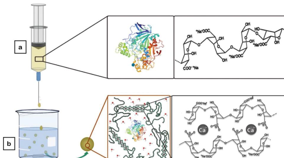
Fig. 1 Schematic representation showing the preparation of CRL encapsulated in Ca-alginate beads: (a) a solution of 5% (w/v) alginate containing CRL ( $2 \text{ mg ml}^{-1}$ ) is dropped into a (b) 2 or 5%  $\text{CaCl}_2$  solution with a residence time of 10, 30 or 60 min.
