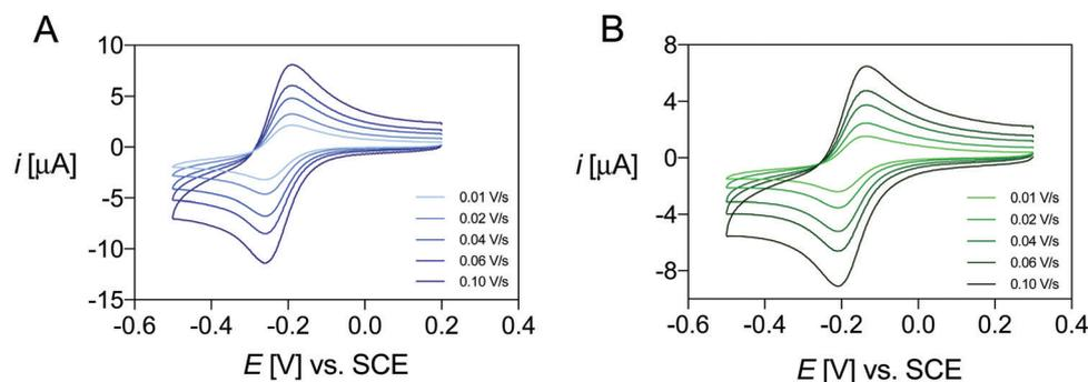
Fig. 5 Representative cyclic voltammograms of the copper complexes of (A) TRI4S ( $C_{\text{Cu}^{2+}} = 8.0 \times 10^{-4} \text{ M}$ ,  $C_{\text{TRI4S}} = 1.0 \times 10^{-3} \text{ M}$ ) and (B) TE4S ( $C_{\text{Cu}^{2+}} = 8.0 \times 10^{-4} \text{ M}$ ,  $C_{\text{TE4S}} = 1.1 \times 10^{-3} \text{ M}$ ) in aqueous solution at physiological pH,  $I = 0.15 \text{ M NaNO}_3$  and  $T = 25 \text{ }^\circ\text{C}$  acquired at different scan rates.
