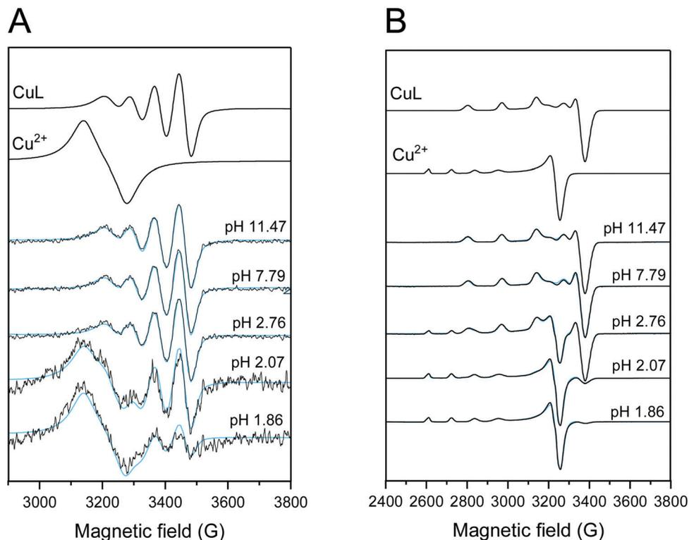
Fig. 4 Experimental (black) and simulated (light blue) EPR spectra of solutions containing  $\text{Cu}^{2+}$  and TE4S ( $C_{\text{Cu}^{2+}} = 8.7 \times 10^{-4}$  M,  $C_{\text{TE4S}} = 1.08 \times 10^{-3}$  M) at (A) room temperature and (B) 77 K. The component spectra obtained from the simulation are shown in the upper part (the spectral intensities were normalized).
