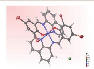
Fig. 1 Molecular structure of complex Fe3a. Ellipsoids are illustrated at 50% probability. Selected bond lengths (Å) and angles (°): Fe(1)-N(5), 1.897(5); Fe(1)-N(4), 1.931(5); Fe(1)-N(3), 1.955(5); Fe(1)-N(1), 1.912(5); Fe(1)-O(2), 1.885(4); Fe(1)-O(3), 1.881(4); O(3)-Fe(1)-N(4), 178.2(2); O(2)-Fe(1)-N(3), 178.6(2); O(2)-Fe(1)-O(3), 88.97(18); O(2)-Fe(1)-N(5), 88.27(18); O(3)-Fe(1)-N(5), 95.64(18); N(3)-Fe(1)-N(5), 91.9(2); N(1)-Fe(1)-N(5), 175.3(2); N(4)-Fe(1)-N(5), 84.6(2).
