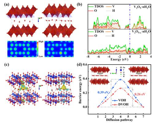
Fig. 4 (a) Optimized crystal structure of VOH and DVOH and corresponding charge distribution sliced along the (00I) direction. (b) Calculated DOS of the VOH and DVOH. (c) Charge density difference of the Zn/VOH and Zn/DVOH (yellow areas: electron depletion. Light blue areas: electron accumulation). The isosurface is set to be 0.005 e  $Å^{-3}$ . (d) Diffusion barrier profiles of  $Zn^{2+}$  transport in DVOH and VOH nanosheets along the b axis (insets show the Zn<sup>2+</sup> diffusion process).
