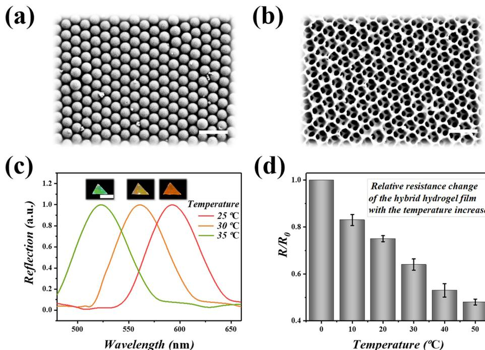
Fig. 2 Characterization of graphene hybrid structural color hydrogels. (a) The SEM image of the colloidal crystal template. (b) The SEM image of the inverse-opal structured hydrogel film. Scale bars in (a and b) are 500 nm. (c) Inverse-opal images and the relationship between the reflectance wavelength and the temperature. Scale bar in (c) is 1 cm. (d) Relative resistance changes with the increase of temperature.
