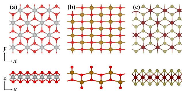
Fig. 1 Top (upper) and side (lower) views of the atomic configurations of three magnetic 2D monolayers: (a) CoO<sub>2</sub>, (b) FeO<sub>2</sub>, and (c) VTe<sub>2</sub>.
