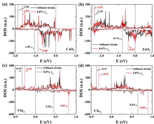
Fig. 5 DOS (in units of a.u.) of spin-up (top) and spin-down (bottom) for the metal atoms (Co, Fe and V) of (a)  $\text{CoO}_2$ , (b)  $\text{FeO}_2$ , (c)  $\text{VSe}_2$  and (d)  $\text{VTe}_2$  monolayers without strain and under the biaxial tensile strain that leads to the lowest overpotential. Here, the red and black dashed lines denote the d-band centers of spin-up and spin-down for the metal atoms, and the Fermi level is set to zero.
