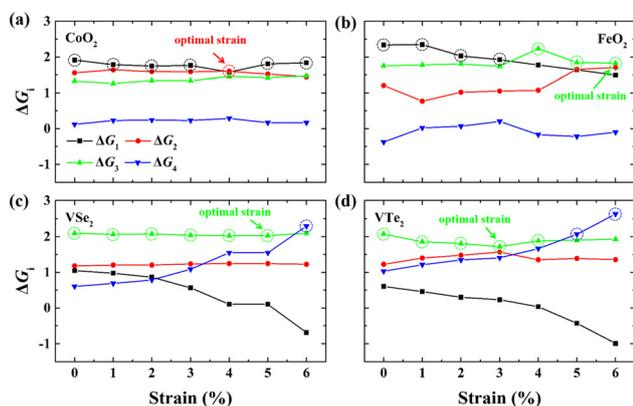
Fig. 3 Gibbs free energy differences ( $\Delta G_i$ ) in the elementary reaction steps for (a)  $\text{CoO}_2$ , (b)  $\text{FeO}_2$ , (c)  $\text{VSe}_2$  and (d)  $\text{VTe}_2$  monolayers under different biaxial tensile strains. The PDSs are circled by dash lines and the optimal strains for the lowest overpotentials are marked by arrows.
