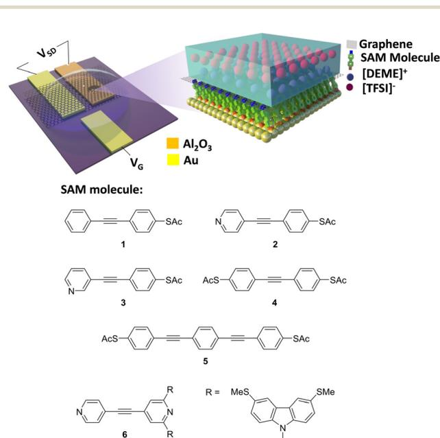
Fig. 1 Experimental setup (top) and molecules measured in this work (bottom) (synthesis and characterizations of 1–3 and 6 were reported previously,<sup>57</sup> synthesis and characterizations of 4 and 5 are reported in the ESI<sup>†</sup>).
