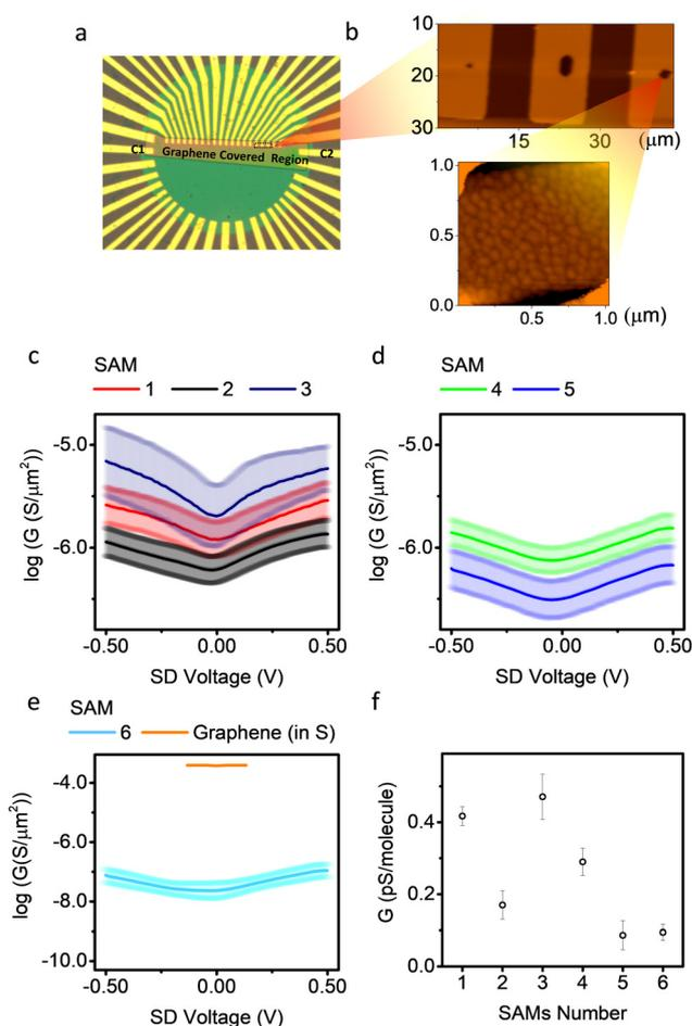
**Fig. 3** (a and b) Optical micrographs of a typical micro-well-based device used in this work. (c–e) Conductance  $G$  on a log scale vs. applied source-drain voltage for SAMs **1–5**, and in-plane conductance across graphene. (f) Zero-bias conductance of molecules **1–6**.
