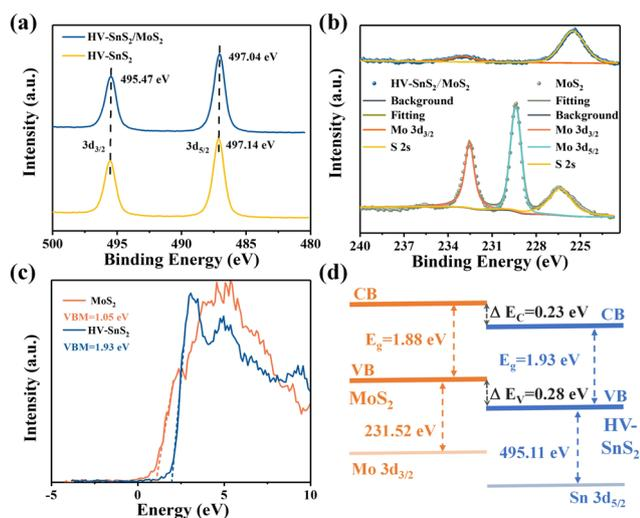
Fig. 4 (a) XPS spectra of Sn 3d<sub>3/2</sub> and Sn 3d<sub>5/2</sub>. (b) XPS spectra of Mo 3d<sub>3/2</sub> and Mo 3d<sub>5/2</sub>. (c) VB spectra and VBM fitting of HV-SnS<sub>2</sub> and MoS<sub>2</sub>. (d) Band alignment information of HV-SnS<sub>2</sub>/MoS<sub>2</sub>.
