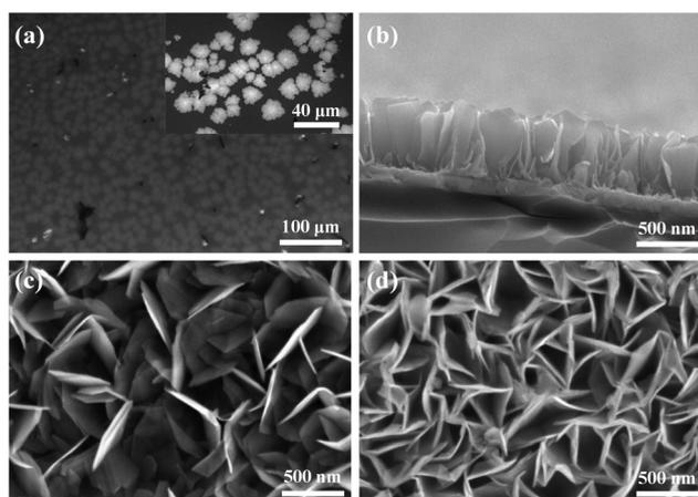
Fig. 2 (a) Top optical image of the MoS<sub>2</sub> nanosheets. The inset is a high magnification optical image. (b) Sectional-view SEM image of HV-SnS<sub>2</sub>. (c) Top SEM image of LV-SnS<sub>2</sub>/MoS<sub>2</sub>. (d) Top SEM image of HV-SnS<sub>2</sub>/MoS<sub>2</sub>.
