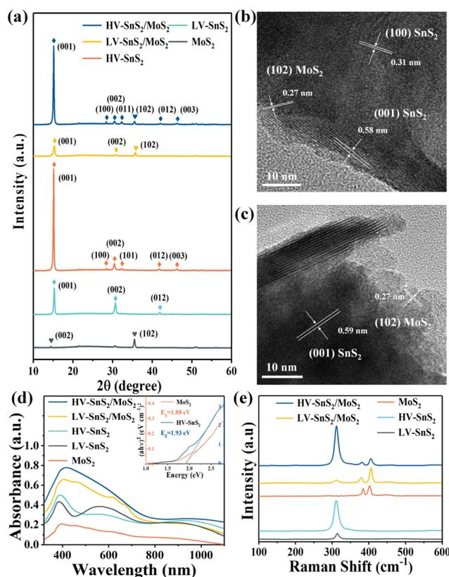
Fig. 3 (a) XRD pattern of HV-SnS<sub>2</sub>/MoS<sub>2</sub>, LV-SnS<sub>2</sub>/MoS<sub>2</sub>, HV-SnS<sub>2</sub>, LV-SnS<sub>2</sub>, and MoS<sub>2</sub>. (b) TEM image of HV-SnS<sub>2</sub>/MoS<sub>2</sub>. (c) TEM image of LV-SnS<sub>2</sub>/MoS<sub>2</sub>. (d) UV-Vis absorption spectroscopy of all samples. The inset is Tauc plot for estimating the bandgap energies ( $E_g$ ) of MoS<sub>2</sub> and HV-SnS<sub>2</sub>. (e) Raman spectra of all samples.
