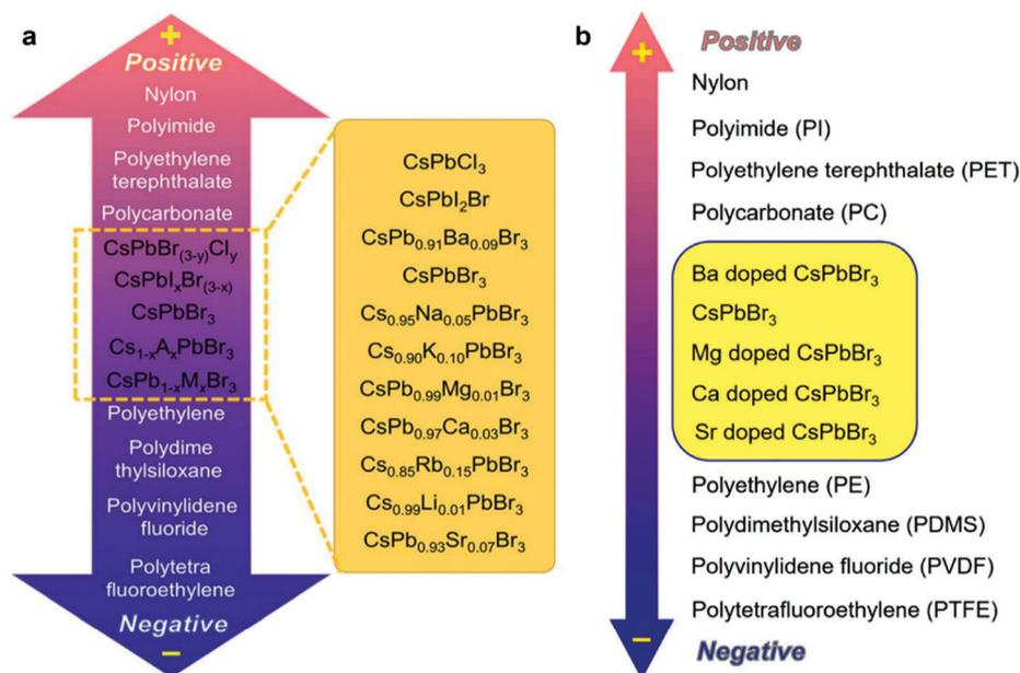
Fig. 7 Triboelectric series of  $\text{CsPbBr}_3$  perovskite and its Cs-site and Pb-site substituted compounds. Qualitative triboelectric series of the (a) pristine  $\text{CsPbBr}_3$ ,  $\text{Cs}_{1-x}\text{A}_x\text{PbBr}_3$  and (b)  $\text{CsPb}_{1-x}\text{M}_x\text{Br}_3$  perovskites. Reproduced with permission from ref. 87 and 90. Copyright 2020 from Elsevier and Copyright 2020 from Royal Society of Chemistry.
