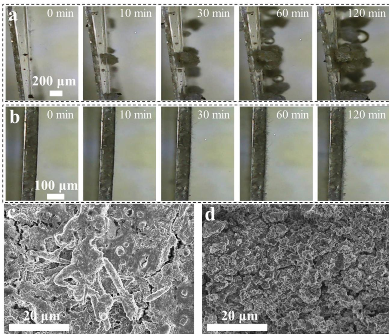
Fig. 4 The *in situ* optical photograph of the Na plating process on the surface of the (a) bare Na and (b) Na/VN electrode. The SEM images of the (c) bare Na and (d) Na/VN electrodes after 10 cycles at  $0.5 \text{ mA cm}^{-2}$  with  $1 \text{ mA h cm}^{-2}$ .
