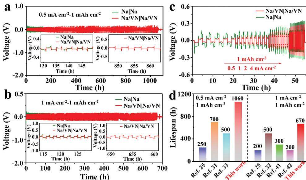
Fig. 2 Galvanostatic cycling of bare Na and Na/VN electrodes in symmetric cells (a) at  $0.5 \text{ mA cm}^{-2}$  with  $1 \text{ mAh cm}^{-2}$  and (b) at  $1 \text{ mA cm}^{-2}$  with  $1 \text{ mAh cm}^{-2}$ . (c) Rate performance of Na/VN and bare Na symmetric cells at various current densities of  $0.5\text{--}4 \text{ mA cm}^{-2}$ . (d) A comparison of the lifespan of Na/VN with the previously reported Na metal anodes.
